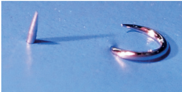
Fig 6. The exterior profile of a barb vs a helical staple exiting an artificial vessel model.
