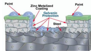
Damaged Zinc / Paint Coating As long as any zinc is present no steel can rust or erode.
