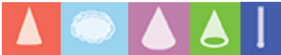
Figure 33: Spray Patterns: Flat Fan, Mist/Fog Fan, Full Cone, Hollow Cone, Straight Jet 27
