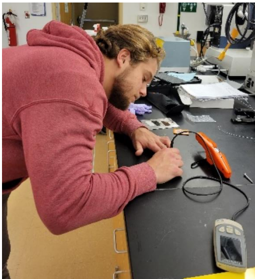
Figure 56: DeFelsko PosiTector in Use
