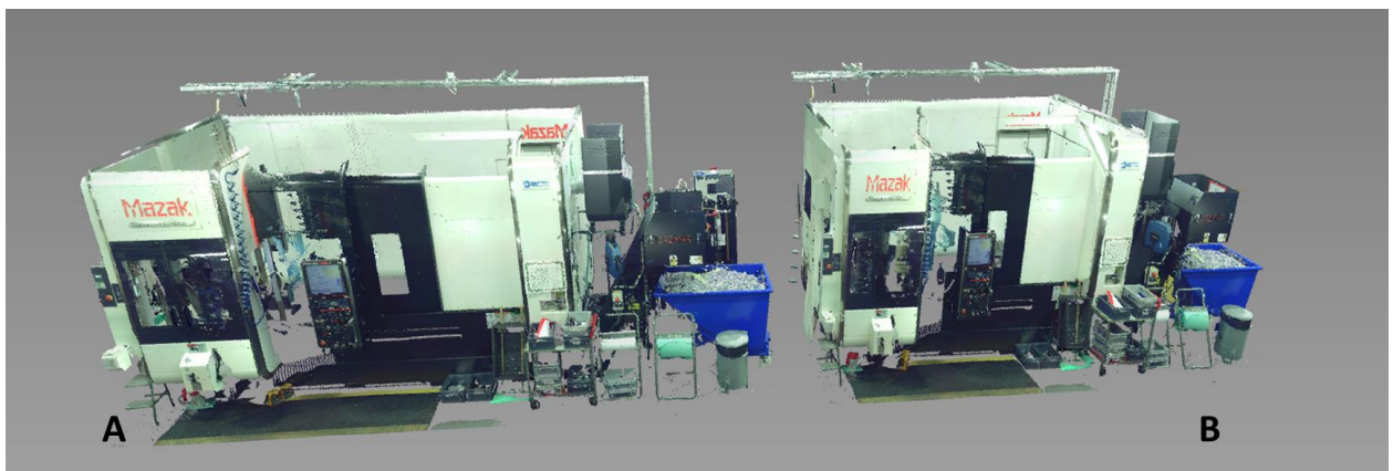
Figure 19: Machine model (left) used to generate models of machinery that were unavailable in 3D CAD (right) via scaling based on 2D drawings.
