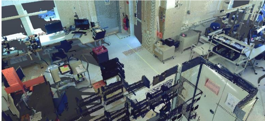
Figure 16: A visualization showing a part of the spatial data gathered via 3D laser scanning.
