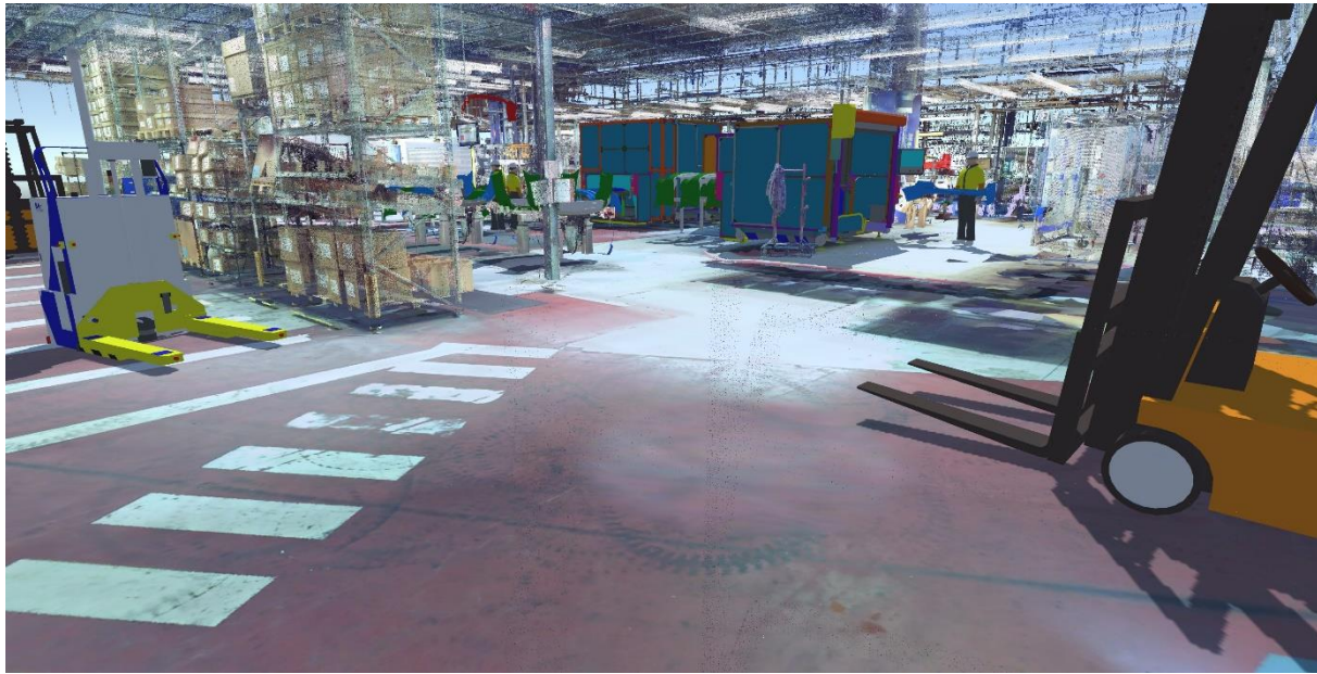
Figure 21: Example of the final model as it would be seen when visualized in immersive VR. The forklifts and operators move around and conduct simulated tasks in the model which consists of a combination of both point cloud and 3D CAD data.
