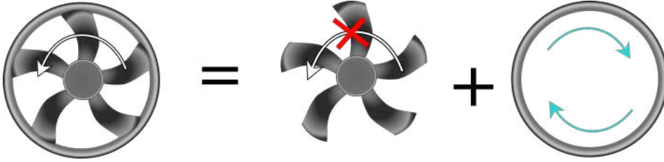
Figure 2.3: Principle of the Multiple Reference Frame approach: the blade geometry is stationary, while the relative velocities are transformed into a rotating reference frame with the opposite sense of rotation.
