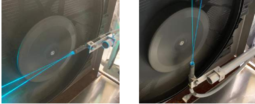
Figure 4.4: Positioning of the 2D LDA probe in the test section. Left: x - and z -component, right: x - and y -component of the velocity vector are measured.
