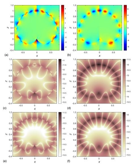
Fig. 6 Field images for scattering from the "tomato" in the plasmonic case and with  $E^{\rm in}(r) = x e^{{\rm i}5z}$ : (a, c, e) the scattered/transmitted  $E_{\rho}(r,0)$ -field; (b, d, f) the scattered/transmitted  $H_{\theta}(r,0)$ -field; (c,d)  $\log_{10}$  of estimated absolute field error for "HK 8-dens"; (e, f) The same for "Dirac". The colorbar range in (a) is set to [-4.55, 4.55]
