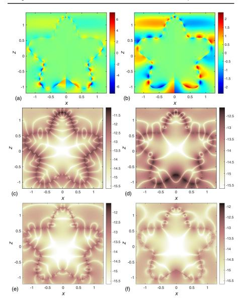
Fig. 4 Field images for scattering from the "rotated starfish" in the plasmonic case and with  $E^{\rm in}(r) = xe^{\rm i6z}$ : (a, c, e) the scattered/transmitted  $E_{\rho}(r,0)$ -field; (b, d, f) the scattered/transmitted  $H_{\theta}(r,0)$ -field; (c, d)  $\log_{10}$  of estimated absolute field error for "HK 8-dens"; (e, f) the same for "Dirac"
