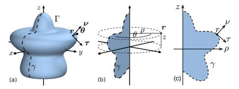
**Fig. 2** Notation for an axially symmetric surface  $\Gamma$  generated by a curve  $\gamma$ : (a) a point r on  $\Gamma$  has outward unit normal v and unit tangent vectors  $\tau$  and  $\theta$ ; (b) cylindrical coordinates  $(\rho, \theta, z)$  of r; (c) coordinate axes and vectors in the half-plane  $\mathbb A$  defined by  $\theta=0$
