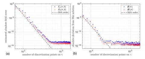
Fig. 5 Convergence as a function of the number of discretization points on  $\gamma$  of: (a) the scattered/transmitted  $E_{\rho}(\mathbf{r},0)$ -field and  $H_{\theta}(\mathbf{r},0)$ -field, shown in Fig. 4e, f; (b) the scattered/transmitted  $E(\mathbf{r})$ -field and  $H(\mathbf{r})$ -field resulting from the incident field (56) and  $\Gamma$  being the unit sphere
