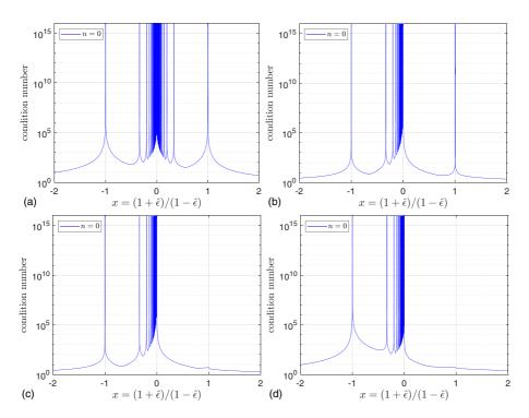
Fig. 10 The unit sphere. Condition numbers of system matrices of the discretized modal integral equations (55) with azimuthal index n=0 in the quasi-static limit  $k_+=k_-=0$ . The plasmonic case is  $x \in (-1,1)$  and the positive dielectric case is  $x \in (-2,-1) \cup (1,2)$ . (a) "HK 8-dens"; (b) "Dirac"; (c) The "Dirac" (5:8,5:8) diagonal block; (d) The "Dirac" version (51)
