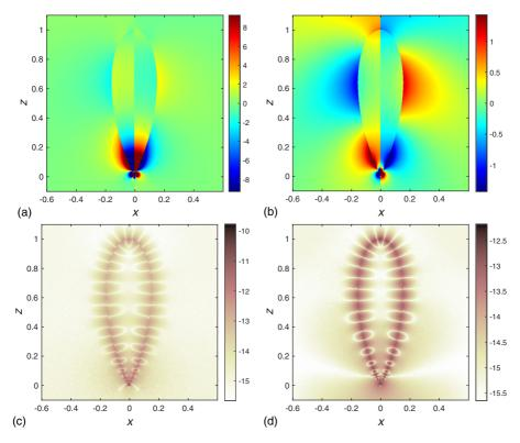
Fig. 8 Field images for scattering from the "drop with a sharp tip" in the plasmonic case and with  $E^{\rm in}(r) = xe^{{\rm i}5z}$ : (a,c) the scattered/transmitted  $E_\rho^\downarrow(r,0)$ -field; (b, d) the scattered/transmitted  $H_\theta^\downarrow(r,0)$ -field; (c, d)  $\log_{10}$  of estimated absolute field error for "Dirac". The colorbar range in (a) is set to [-9.27, 9.27] and in (b) set to [-1.43, 1.43]
