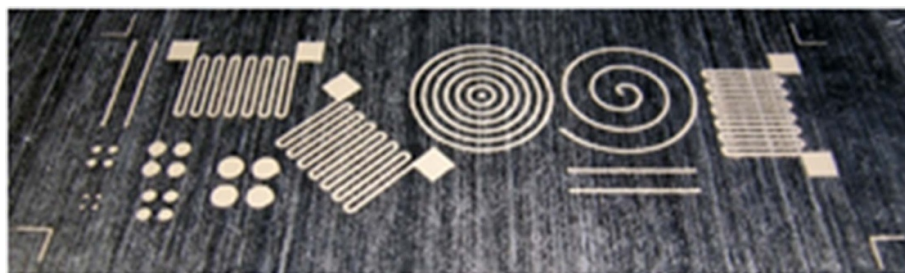
Figure 10. Complex shapes made with screen-printed silver paste.
