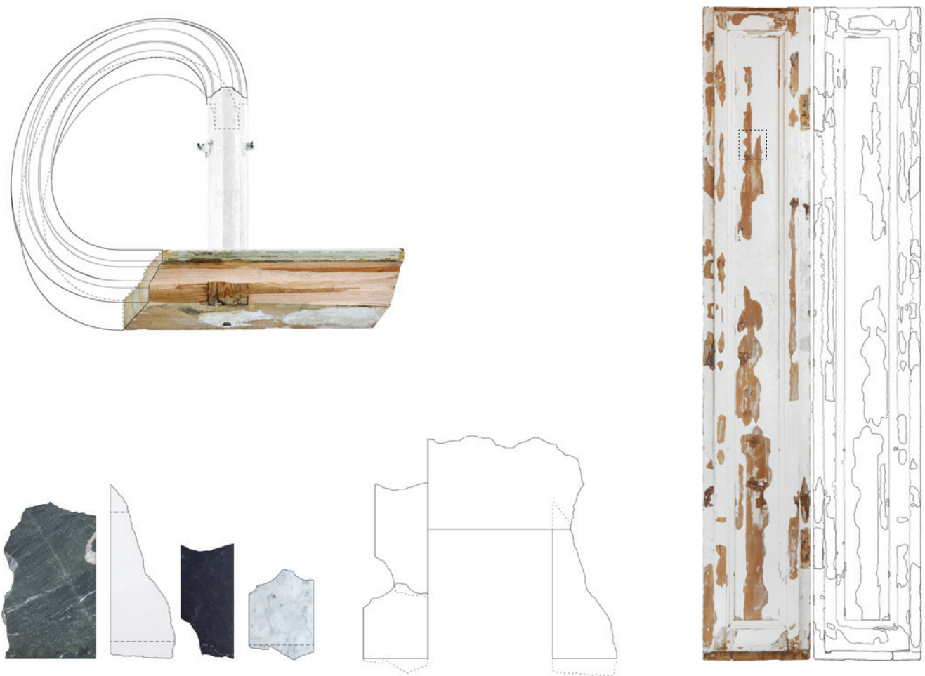
11 Window frame: Isometric of digital model obtained with photogrammetry (top left). Door panel: Elevation of digital model obtained with photogrammetry (right). Marble sheets: Elevation of photographed sheets assembled into mantelpiece, with trimmed parts indicated with dashed lines (bottom left).
