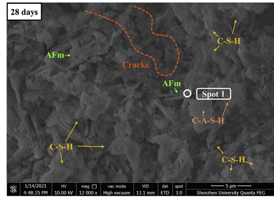
(a) Microstructure of the LC3-PP-ECCs after curing for 28 d
