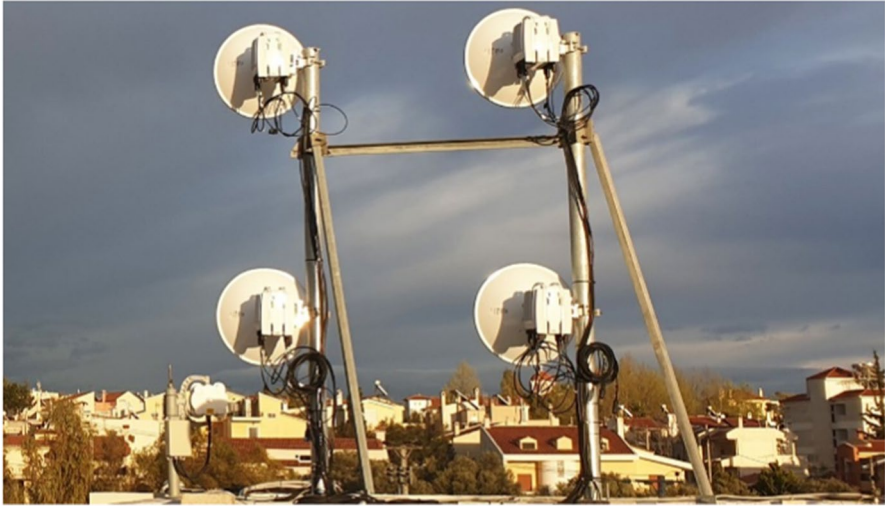
Fig. 1 Ericsson demonstrator of LOS-MIMO at 70 GHz band [5]
