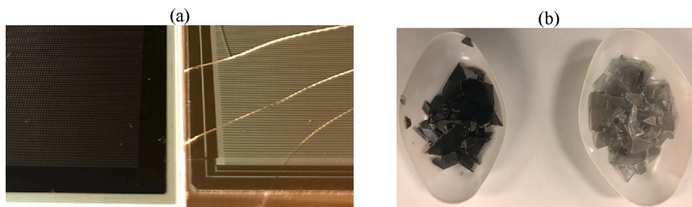
Fig. 1. Front and back side of the LCD before (a) and after (b) the removing of the organic layer. Dark: front side, bright: back side.
