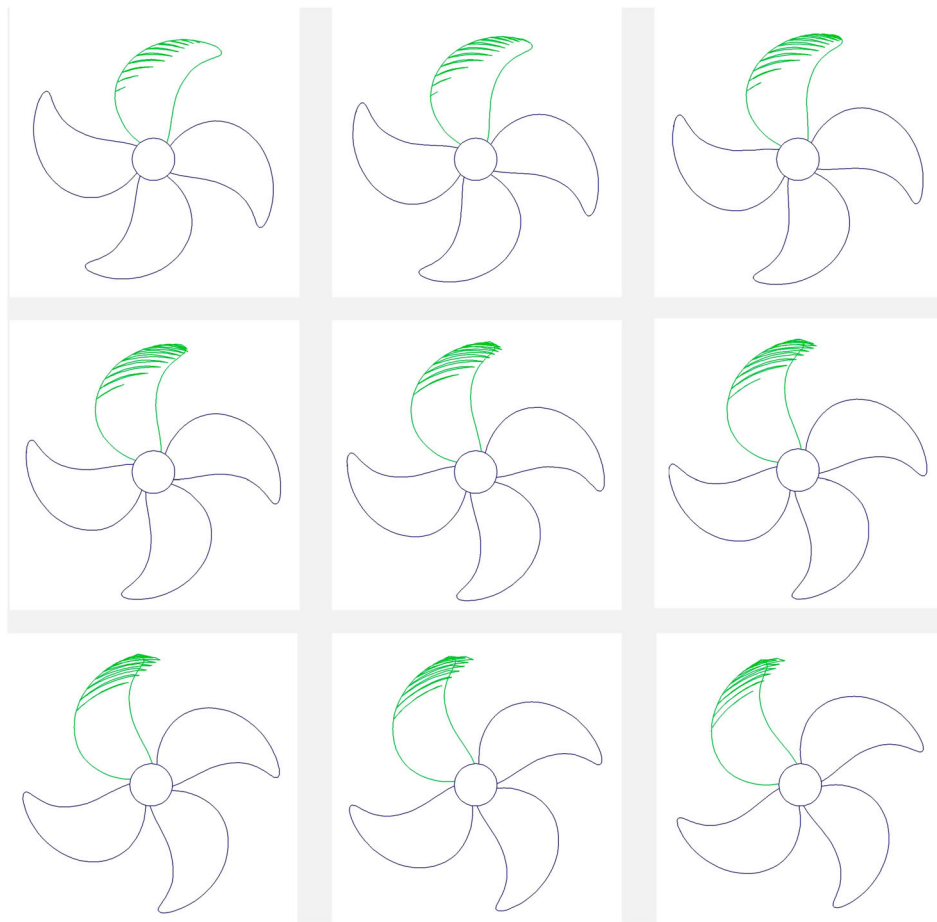
Figure 5. Cavity shape on blade in 9 time steps.
