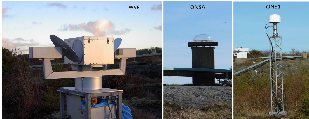
Figure 3. The water vapour radiometer (WVR) and GNSS stations (ONS1 and ONSA) at the Onsala Space Observatory.
