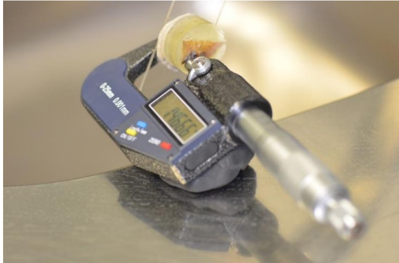
Figure 8: Micrometer with a reading of 25\text{mm} \pm 0.001\text{mm} used for measurements according to Fig. 9 and for control of parallelism.
