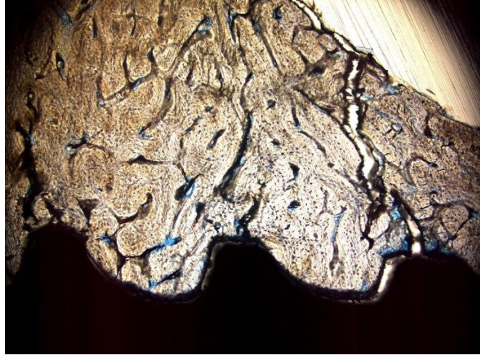
Figure 22: Partially detached bone from the implant surface because of the shear forces the specimens were exposed to during the preparation; Specimen # 35.
