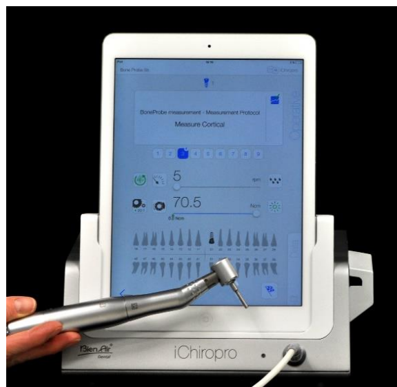
Figure 3: BoneProbe in the development status as used in this study. A surgical contra angle has been modified to house the BoneProbe mechanism while the drill unit can be used for monitoring the torque required for a certain level of expansion.
