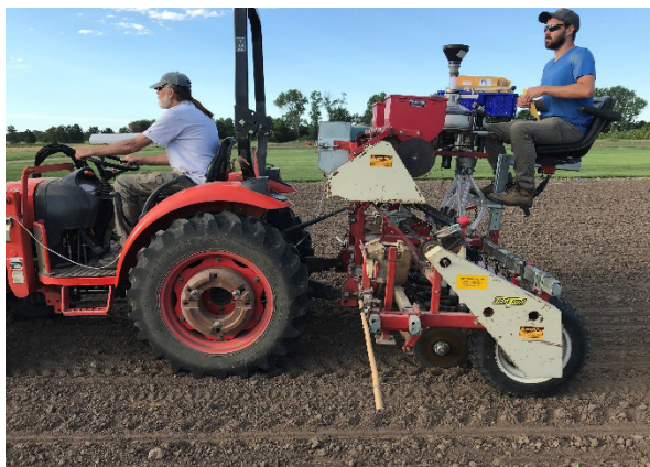
Figure 1. Hege 1000 grain drill for planting hemp variety plots.
