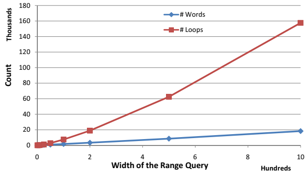
Figure 4.1. The effect of rocket query range width. The Y axis shows the number of iterations of the inner loop of the OR code (upper line), and the number of words read from the original and intermediate-result bit vectors (lower line). The X axis shows the width of the query range.
