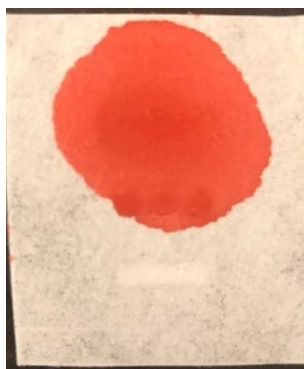
Figure 4.3- This image shows the backside of the splitting layer after dissection of the failed \mu PAD during the “water test”. This \mu PAD used PVC-based plastisol ink.
