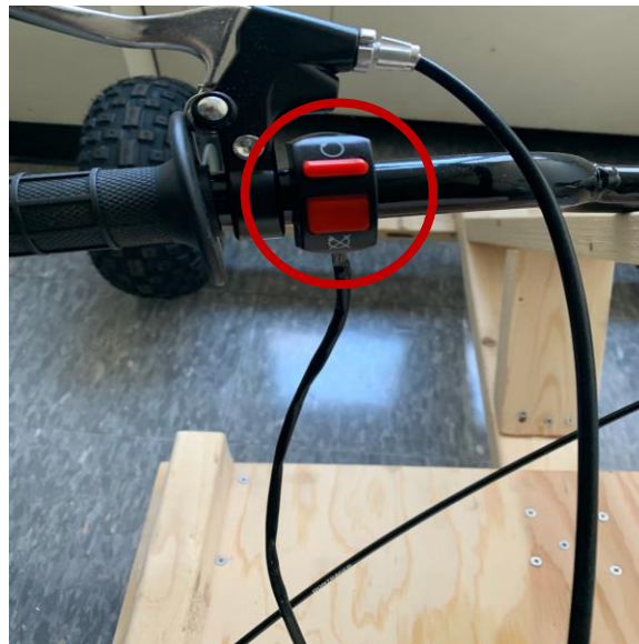
Figure 3.9.3 Kill switch mounted on handlebar
