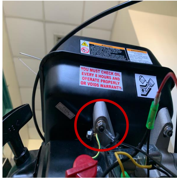
Figure 3.9.2 Grounding the switch
