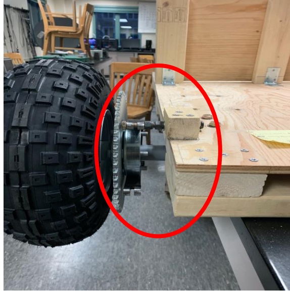
Figure 3.6.1 Brake band attached to kart
