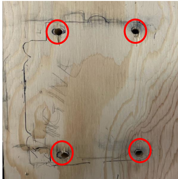
Figure 3.3.1 Engine's outline with fastening holes marked and drilled.
