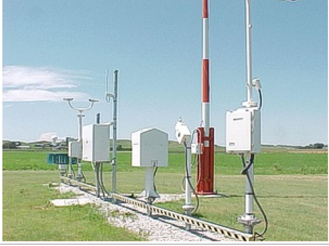
**Figure 2.** Above is a photograph of ASOS equipment recording weather data provided by NWS and NOAA. This equipment is located in the Raleigh area and runs non-stop, updating weather observations every minute 24 hours a day. The ASOS network has more than double the number of full-time service surface weather observing locations in the NWS Raleigh Country Warning Area.
