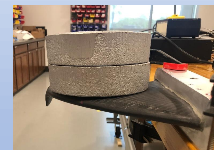
Figure 3: 20 lb. static load applied to the pressure surface of the WF while installed in mounting block.
