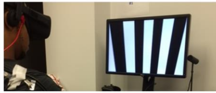
Participant wearing EOG electro-oculogram electrodes and the VR OKN head mounted display while the B&W stripes rotate around them. The image on the screen is a 2D representation of the 3D HMD.
