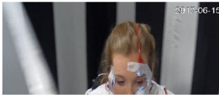
Participant wearing EOG electro-oculogram electrodes sitting in the Drum OKN device while the B&W stripes rotate around them.
