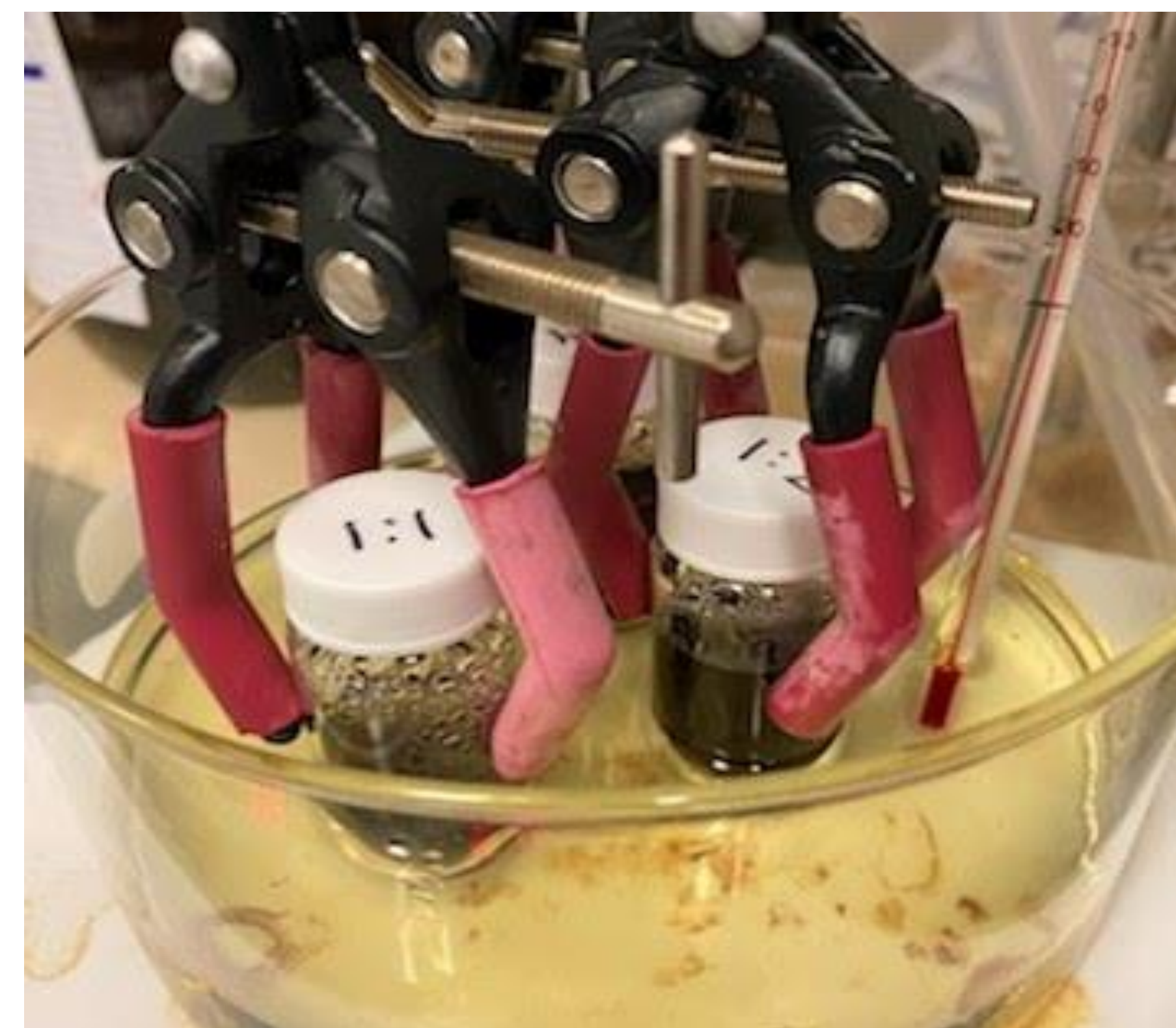
Fig 3: Experimental setup of MNP synthesis with different ratios of dopamine hydrochloride and sodium hydroxide in oil bath. The change in concentration of the dopamine hydrochloride and sodium hydroxide 1:1, 1:2, 1:4 ratios is being studied. A change in color from clear (beginning of reaction) to black (end of the reaction, 3 hours) was observed.
