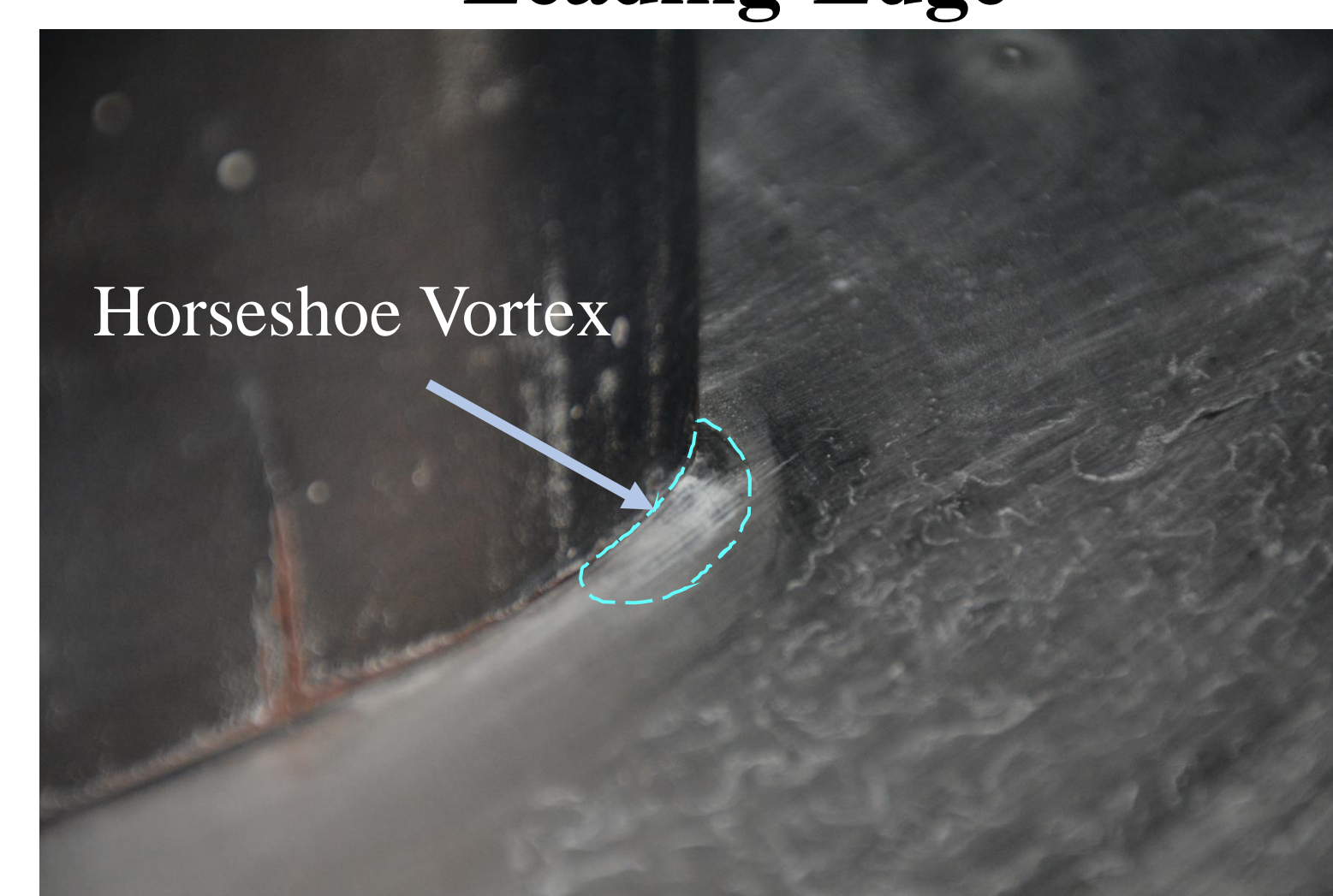
Figure 4a: Horseshoe vortex visualization from case five.
