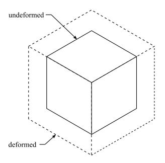
Fig. 3.4 A three-dimensional body subjected to isotropic expansion.
