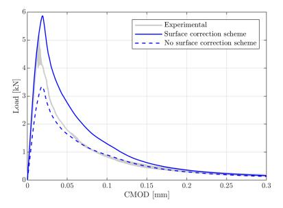
Fig. 5.11 Load-CMOD response for the unnotched beam (d = 50 mm) using a trilinear constitutive law with and without surface correction factors.
