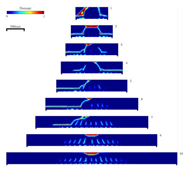
Fig. 7.7 Numerical fracture pattern at failure using the normal mesh. The cross-section is taken through a reinforcing bar
