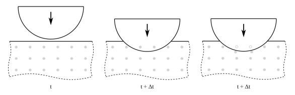
Fig. 4.9 Development of a contact surface between a rigid penetrator and deformable body. Displacement of a particle is equal to the length of the shortest path between the particle and penetrator surface.
