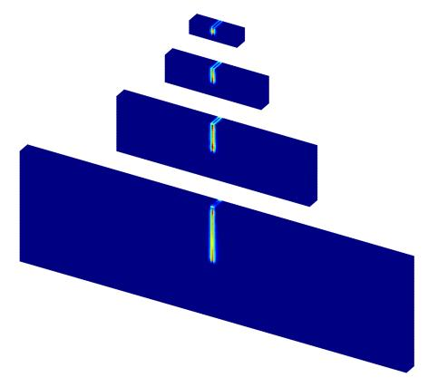
Fig. 6.2 Numerical softening damage for the half-notched specimens
