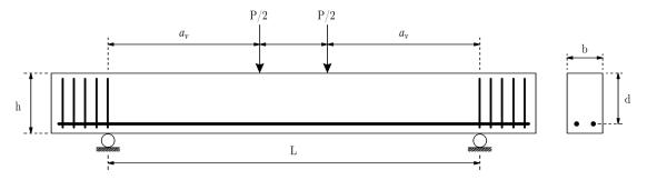
Fig. 2.6 Typical four-point bending test setup
