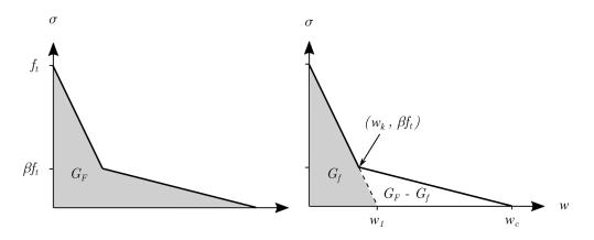
Fig. 5.5 Bilinear tension softening constitutive law ( $\sigma$ -w). Adapted from [10, 236].
