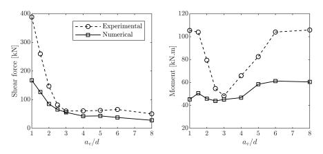
Fig. 7.6 Shear force and moment at failure against  $a_v/d$
