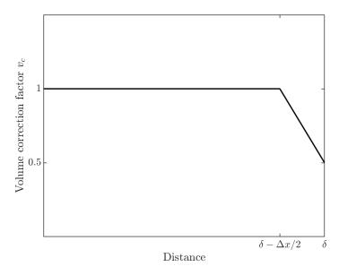
Fig. 4.5 Volume correction factor  $v_c$  against distance
