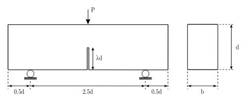
Fig. 5.8 Schematic of the experimental setup. Adapted from Grégoire et al. [98].
