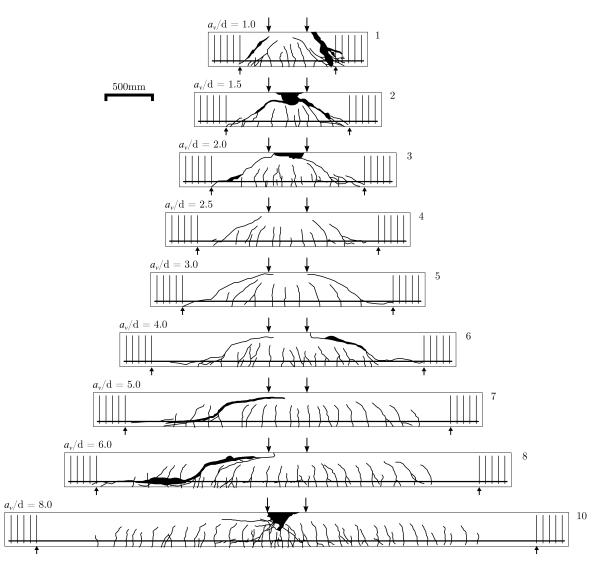
Fig. 7.5 Failure behaviour in beams tested by Leonhardt and Walther [135]. Refer to Table 7.1 for dimensions.
