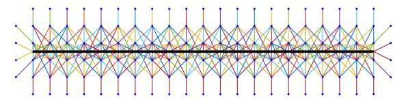
Fig. 5.19 Bonds that cross the theoretical unit fracture surface centred within a  $5m \times 5m \times 5m$  cube ( $\Delta x = 50$  mm)
