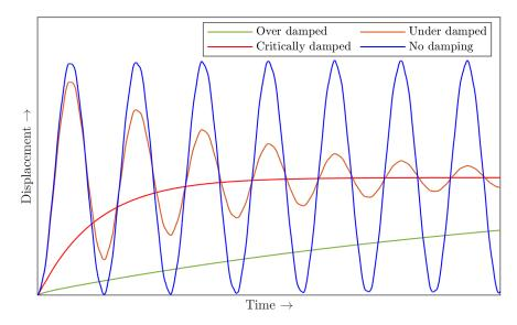
Fig. 4.7 Influence of the local damping coefficient on the convergence speed for load-controlled quasi-static analysis
