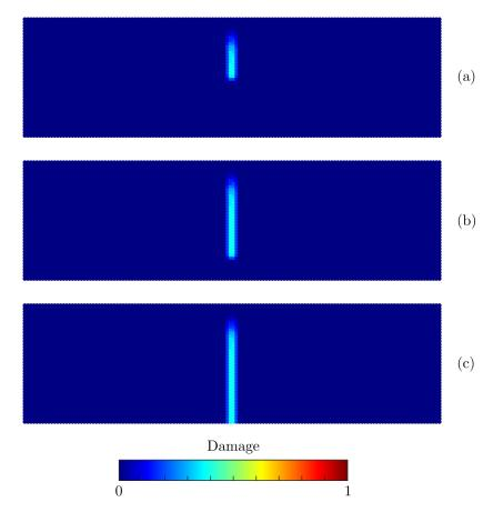
Fig. 5.23 Numerical fracture path at 0.5 mm of applied displacement. The residual load carrying capacity is approximately 30 N for each member. (a) half-notched, (b) fifth-notched, (c) unnotched.
