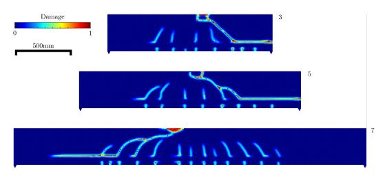
Fig. 7.8 Numerical fracture pattern at failure for Beam 3, 5, and 7 using the fine mesh
