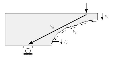
Fig. 2.7 Shear transfer actions in a reinforced concrete member: compressive strut  $V_{cs}$ , uncracked compressive zone  $V_c$ , aggregate interlock  $V_a$ , dowel actions  $V_d$ .
