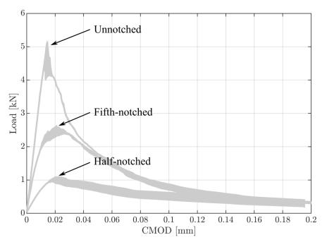
Fig. 5.9 Load-CMOD response for Beam 4 (d = 50 mm): unnotched, fifth-notched, and half-notched [98]
