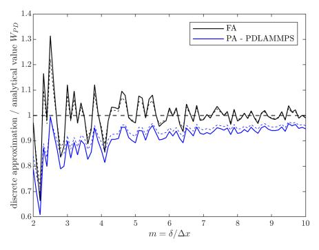
Fig. 5.13 *m*-convergence of the discrete strain energy density approximation.  $\Delta m = 0.1$
