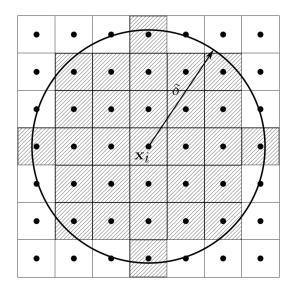
Fig. 4.3 Illustration of spatial integration using the meshfree method proposed by Silling and Askari [207]. The hashed areas highlight the computed area
