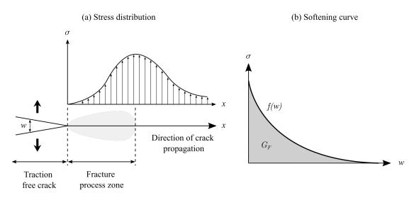
Fig. 2.4 Schematic of the cohesive zone at the crack tip and the traction-separation law ( $\sigma$ -w relationship)
