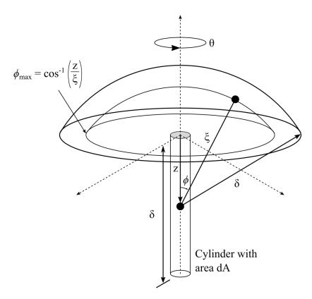
Fig. 3.8 Schematic of the energy release rate  $G_0$  computation
