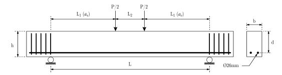
Fig. 7.3 Experimental setup.  $L_1$  is the shear span  $a_v$ . Adapted from Leonhardt and Walther [135].
