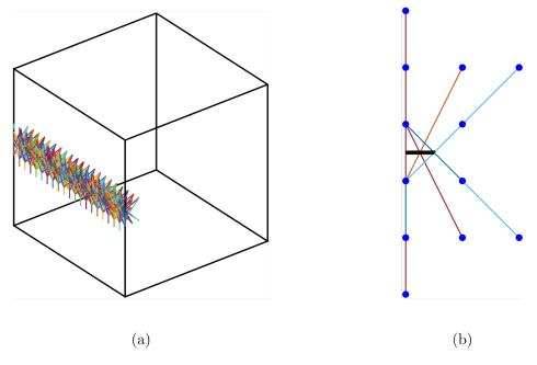
Fig. 5.20 Bonds that cross a theoretical fracture surface at the edge of a peridynamic body
