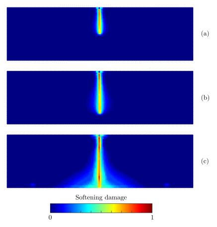
Fig. 5.24 Numerical softening damage at 0.5 mm of applied displacement using the finest mesh  $\Delta x = 1.25$  mm. (a) half-notched, (b) fifth-notched, (c) unnotched.
