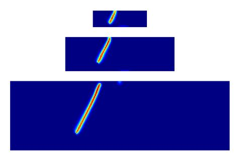
Fig. 6.7 Numerical softening damage for notch eccentricity  $\mu d = 0.625d$ .
