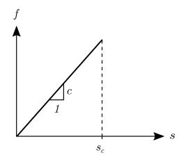
Fig. 3.3 Scalar bond force f as a function of bond stretch s in the linear elastic material model.
