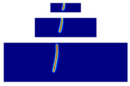
Fig. 6.6 Numerical softening damage for notch eccentricity  $\mu d = 0.3125d$ .
