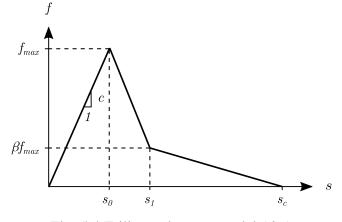
Fig. 5.4 Trilinear damage model (f-s)
