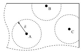
Fig. 4.10 Material point horizons. The horizon of Material Point A is contained completely within the material bulk. The horizon of Material Point B and C lies across the boundary of the peridynamic body.
