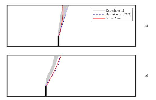
Fig. 6.9 Experimental and numerical crack paths for the mixed mode fracture tests (d = 320mm). Notch eccentricity  $\mu d$ : (a) 0.3125d, and (b) 0.625d
