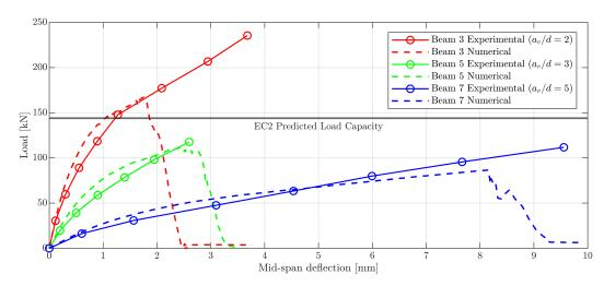
Fig. 7.15 Comparison of experimental and numerical load-displacement curves. The horizontal line indicates the load capacity predicted by EC2.
