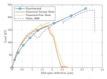
Fig. 7.9 Beam 3 load-displacement curve  $(a_v/d = 2)$
