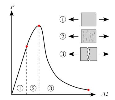
Fig. 5.1 Tensile stress-strain curve for concrete: (1) linear elastic behaviour, (2) development of distributed micro-cracking, (3) localisation of damage and formation of macroscopic cracks.
