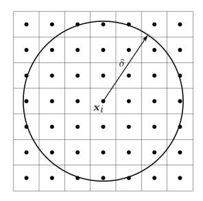
Fig. 4.1 Horizon of node  $\mathbf{x}_i$  in the discretised configuration
