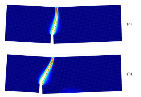
Fig. 5.30 Numerical softening damage for the mixed-mode fracture tests. Notch eccentricity  $\mu d$ : (a) 0.3125d, and (b) 0.625d. Displacement is scaled by a factor of 10.
