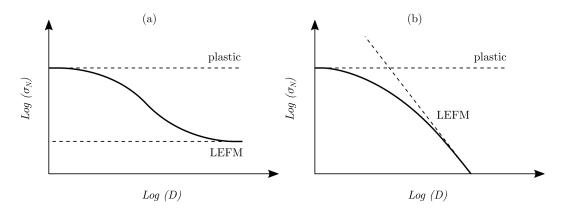
Fig. 6.1 Size effect laws in a log-log scale: (a) Type 1 (unnotched case); (b) Type 2 (notched case). Adapted from Fig. 1 in [216].
