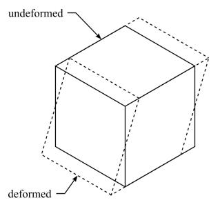
Fig. 3.5 A three-dimensional body subjected to simple shear.
