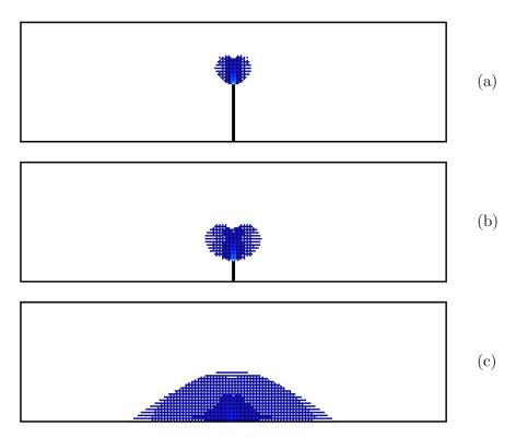
Fig. 5.25 Region of damage energy dissipation at peak load using the finest mesh  $\Delta x = 1.25$  mm. Each point represents the mid-point of a bond that has exceeded the elastic limit. (a) half-notched, (b) fifth-notched, (c) unnotched.
