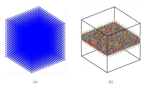
Fig. 5.16 (a) discretised unit cube; (b) all bonds that cross the theoretical unit fracture surface
