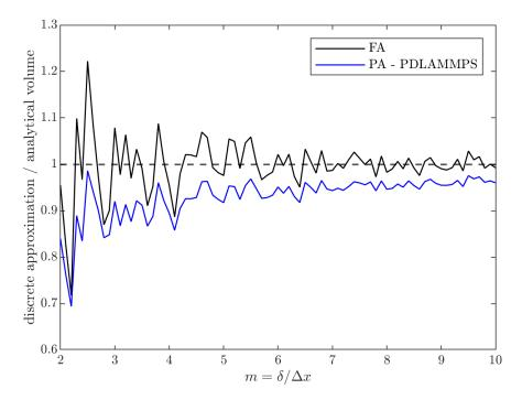
Fig. 5.12 *m*-convergence of the discrete volume approximation.  $\Delta m = 0.1$
