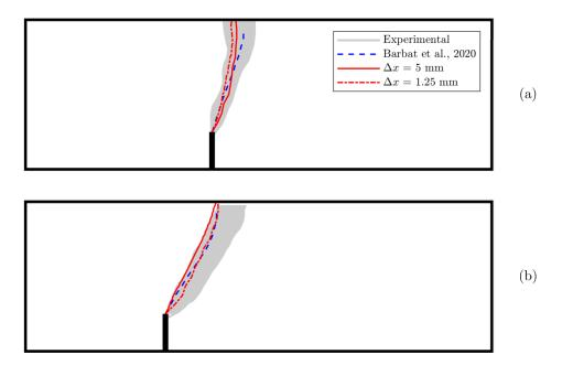
Fig. 5.31 Experimental and numerical crack paths for the mixed-mode fracture tests. Notch eccentricity  $\mu d$ : (a) 0.3125d, and (b) 0.625d
