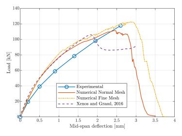
Fig. 7.10 Beam 5 load-displacement curve  $(a_v/d = 3)$
