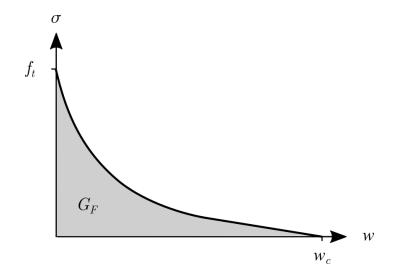
Fig. 5.7 Non-linear tension softening constitutive law ( $\sigma$ -w). Adapted from Fig. 6.1 in Hordijk [115].
