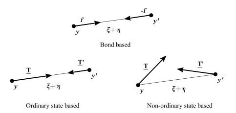
Fig. 3.10 Schematic of bond based, ordinary, and non-ordinary material response. Adapted from Silling et al. [208].
