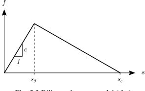
Fig. 5.3 Bilinear damage model (f-s)
