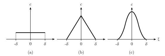
Fig. 3.7 Comparison of influence functions (scale is approximate): (a) constant influence function; (b) triangular influence function (conical); (c) quartic influence function
