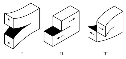
Fig. 2.3 Three principle fracture modes: normal (mode I), in-plane shear (mode II), and out-of-plane shear (mode III).
