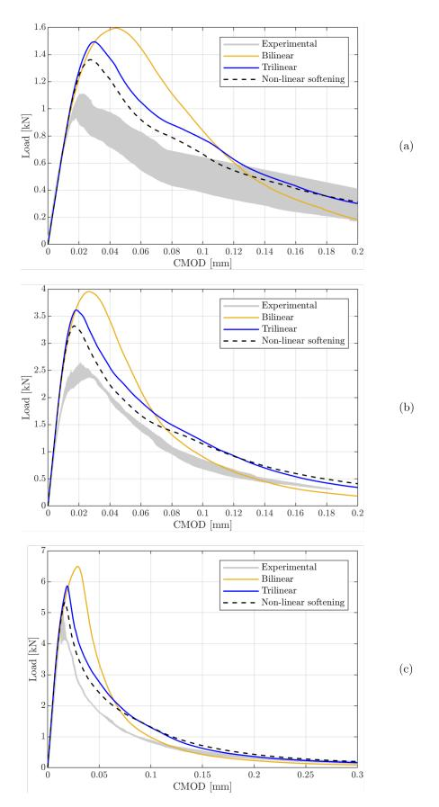
Fig. 5.10 Comparison of load-CMOD results predicted using different constitutive laws: (a) half-notched, (b) fifth-notched, (c) unnotched case.
