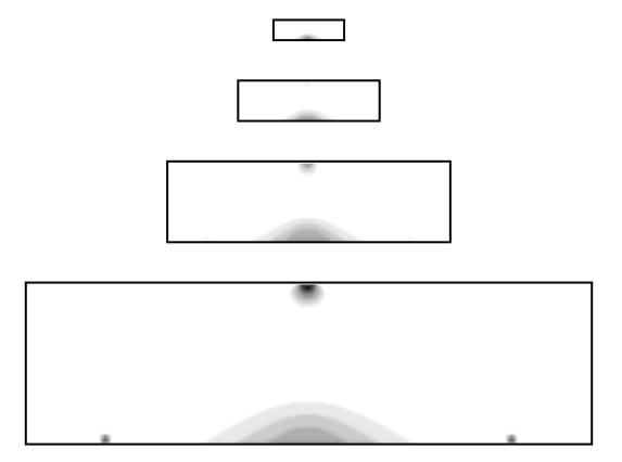
Fig. 6.5 Region of damage energy dissipation at peak load for unnotched members. Mesh resolution  $\Delta x = 5$  mm. Note that a grey colour scale is used to improve the clarity of the figure.
