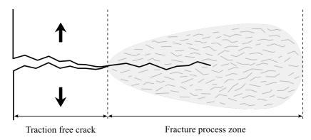
Fig. 2.2 Fracture process zone in a quasi-brittle material.
