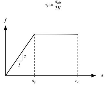
Fig. 7.1 Microplastic Model
