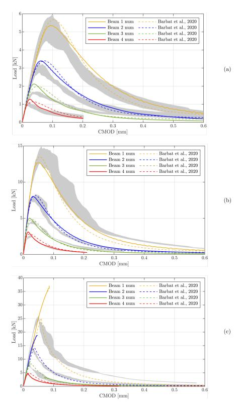
Fig. 6.3 Load-CMOD response for the mode I fracture tests: (a) half-notched, (b) fifth-notched, (c) unnotched case.
