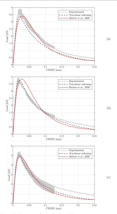
Fig. 5.28 Load-CMOD response for the mixed mode fracture tests. Notch eccentricity  $\mu d$ : (a) 0d, (b) 0.3125d, and (c) 0.625d
