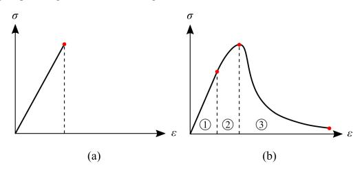
Fig. 2.1 Stress-strain response: (a) perfectly brittle material, (b) quasi-brittle material.
