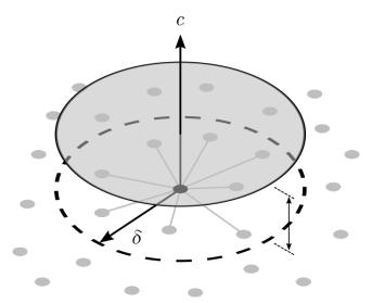
Fig. 3.6 Schematic of a constant influence function for a two-dimensional peridynamic model
