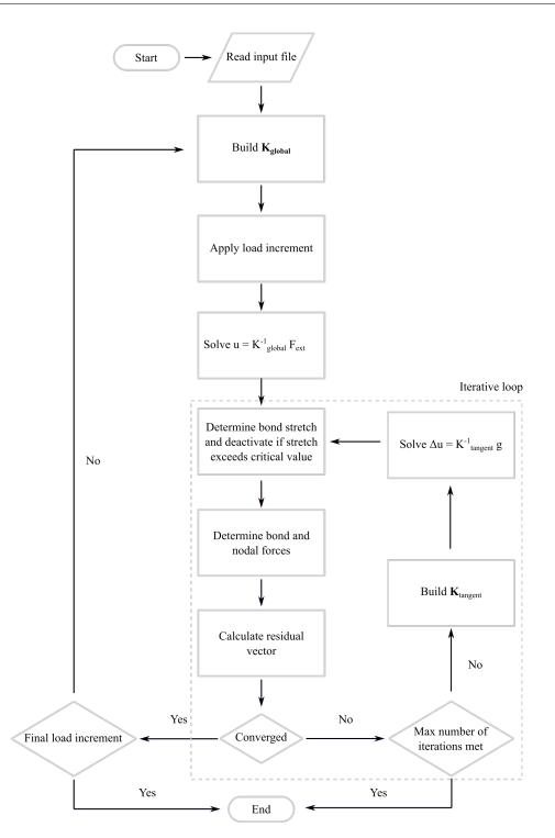
Fig. 4.13 Schematic of an implicit scheme with load-control. After every time *increment* (load step), an *iterative* solution algorithm must be used to determine the equilibrium state, hence the solution process is known as an *incremental-iterative* procedure.
