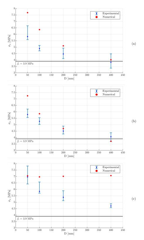
Fig. 6.4 Nominal strength versus depth (characteristic dimension) for the mode I fracture tests: (a) half-notched, (b) fifth-notched, (c) unnotched case. For large unnotched structures, the nominal strength should converge on the tensile strength  $f_t = 3.9$  MPa.
