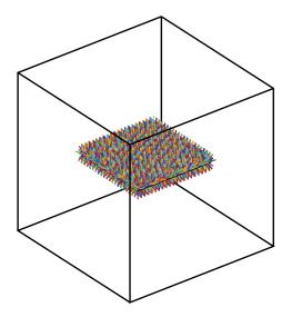
Fig. 5.18 Bonds that cross the theoretical unit fracture surface centred within a  $5m \times 5m \times 5m$  cube. The cube is not drawn to scale.
