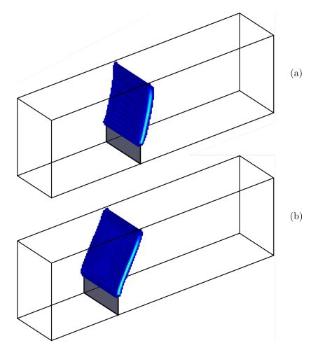
Fig. 5.29 3D crack paths for the mixed-mode fracture tests. Notch eccentricity  $\mu d$ : (a) 0.3125d, and (b) 0.625d
