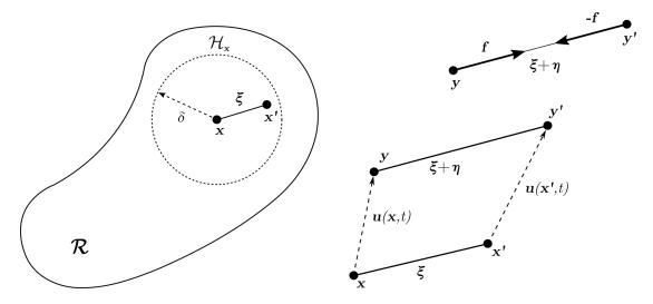
Fig. 3.2 Peridynamic continuum and kinematics of particle pair and bond-based pairwise force function
