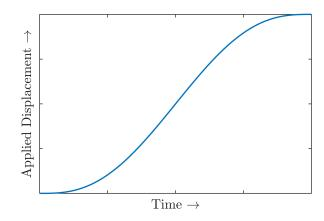
Fig. 4.8 Applied displacement against time using a smooth amplitude curve for displacementcontrolled quasi-static analysis
