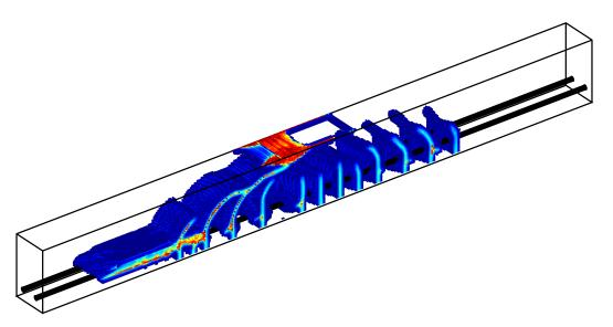
Fig. 7.12 Fracture paths in Beam 7 using the fine mesh
