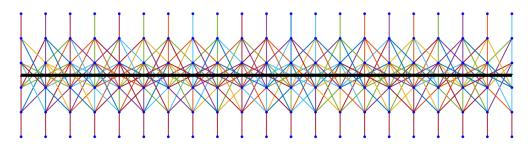
Fig. 5.17 Bonds that cross the theoretical unit fracture surface within a unit cube ( $\Delta x = 50$  mm)
