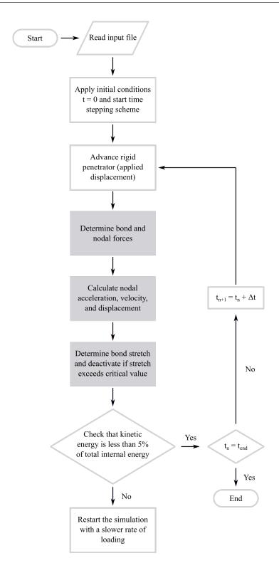
Fig. 4.14 Schematic of a quasi-static explicit solver with displacement-controlled loading
