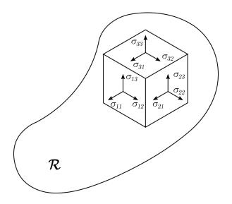
Fig. 3.1 Stress tensor in a continuous solid
