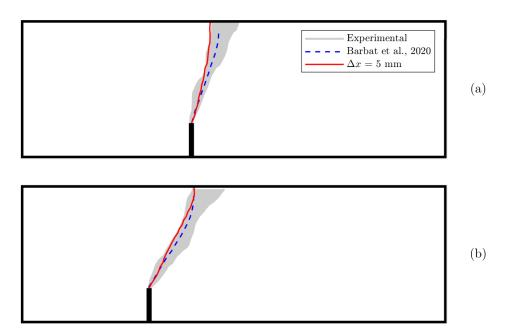
Fig. 6.8 Experimental and numerical crack paths for the mixed mode fracture tests (d = 160mm). Notch eccentricity  $\mu d$ : (a) 0.3125d, and (b) 0.625d
