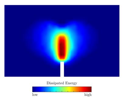
Fig. 5.26 Region of energy dissipation (fracture process zone) at the peak load for the fifthnotched beam.
