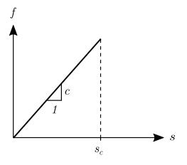
Fig. 5.2 Linear damage model (f-s)
