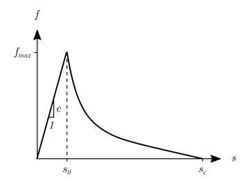
Fig. 5.6 Non-linear damage model (f-s). The force-stretch relationship is described by an exponentially decaying model with a linear term that forces the curve to intersect with the horizontal axis at  $s_c$ .
