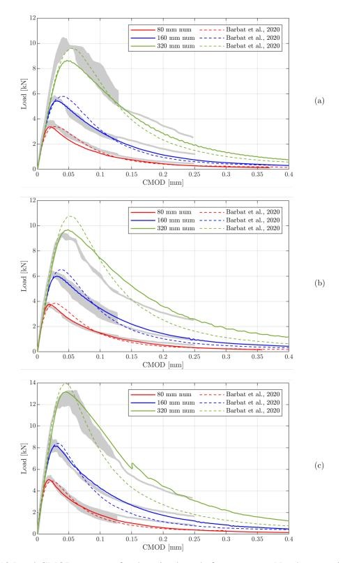
Fig. 6.10 Load-CMOD response for the mixed-mode fracture tests. Notch eccentricity  $\mu d$ : (a) 0d, (b) 0.3125d, and (c) 0.625d
