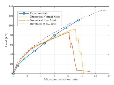
Fig. 7.11 Beam 7 load-displacement curve  $(a_v/d = 5)$
