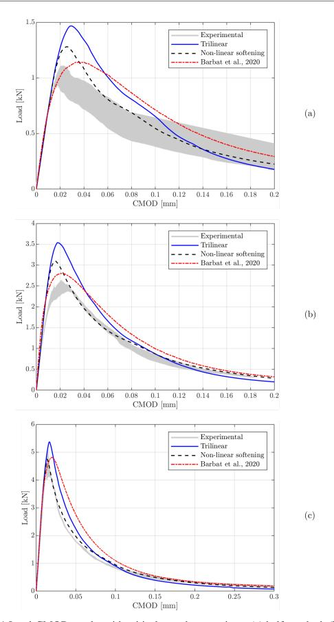
Fig. 5.21 Load-CMOD results with critical stretch corrections: (a) half-notched, (b) fifth-notched, (c) unnotched case.
