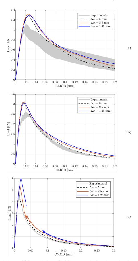
Fig. 5.22 Mesh sensitivity study. Load-CMOD response for three levels of mesh refinement ( $\Delta x = 1.25$  mm, 2.5 mm, and 5 mm). (a) half-notched, (b) fifth-notched, (c) unnotched.
