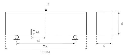
Fig. 5.27 Schematic of the experimental setup. Adapted from García-Álvarez et al. [88].
