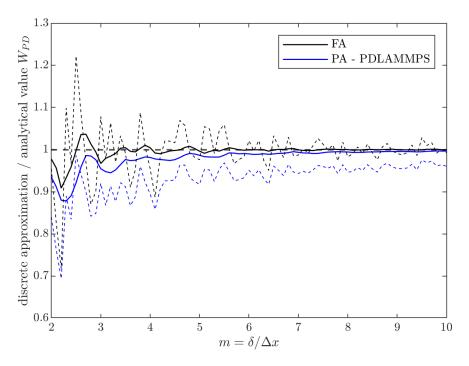
Fig. 5.15 *m*-convergence of the discrete strain energy density approximation using a conical influence function.  $\Delta m = 0.1$
