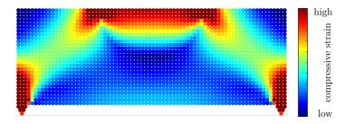
Fig. 7.14 Principal compressive strain distribution in Beam 1. The purpose of this figure is to illustrate the formation of compressive struts and the inclusion of strain values is considered to be redundant.
