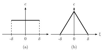
Fig. 5.14 Comparison of micro-modulus functions: (a) constant influence function; (b) triangular influence function (conical)
