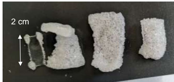
Figure 92: Samples desorbed from 28.5 w/w% methanol content to 10 w/w% and quenched in liquid nitrogen after desorption. Foaming temperatures from left to right: 130, 150, 160, 170 °C.
