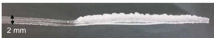
Figure 55: Void development at high concentrations only appearing on the face of the sample that had been in contact with the bottom of the silicone oil bath.
