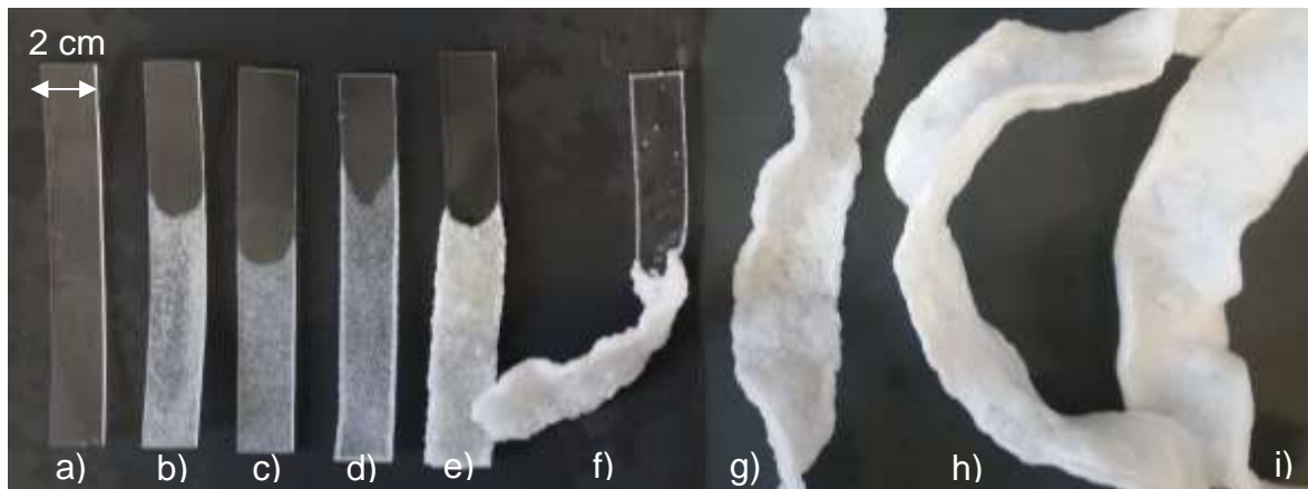
Figure 61: Foaming at 170 °C for 60 s after a liquid nitrogen quench followed by desorption at 25 °C. From left to right the samples contained a) 18.5, b) 17.9, c) 16.9, d) 15.4, e) 13.4, f) 10.4, g) 9.7, h) 9.0, i) 8.7 w/w%. The bottom part is the quenched part.
