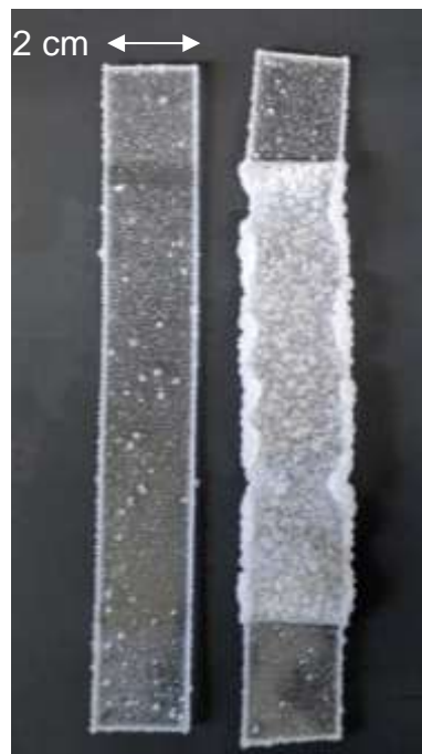
Figure 44: Left: sample subject to yield stress (6 MPa) before desorption to 11.4 w/w%. Right: sample subject to yield stress (25 MPa) after desorption to 11.6 w/w% remaining methanol content.
