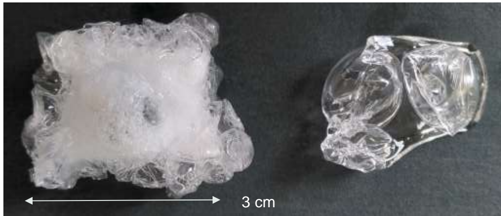
Figure 19: Left: foam formation of fully methanol charged extruded PMMA after a liquid nitrogen quench and transfer to a 170 °C silicone oil bath. Right: foam formation of a fully methanol charged extruded material without a liquid nitrogen quench and transfer to a 170 °C silicone oil bath.
