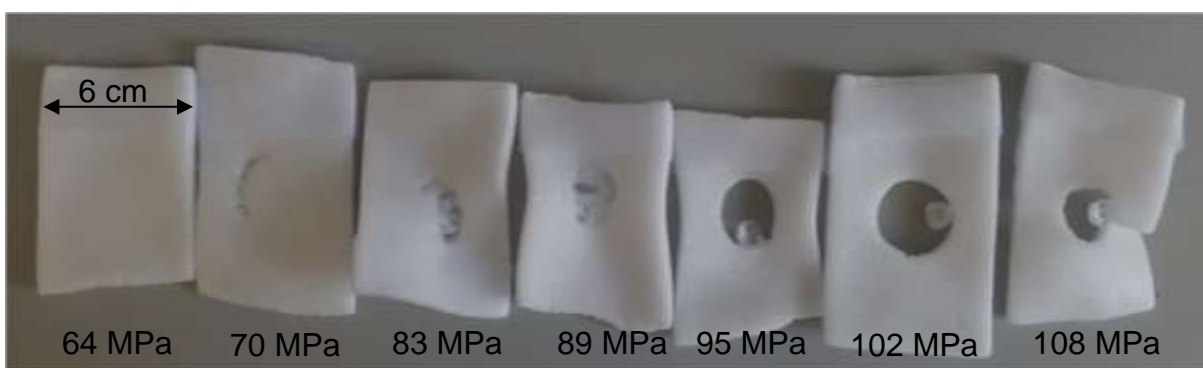
Figure 52: Effect of pre-applied pressure on foaming. From left to right: 64, 70, 76, 83, 89, 95, 102 and 108 MPa of pressure were applied after desorption to under 8 w/w% methanol content. Above 83 MPa almost no voids are created where the pressure was applied.
