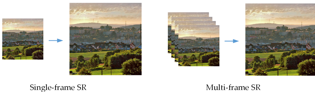
Figure 2.6: Single-frame and multi-frame SR. Source images are obtained from [141].
