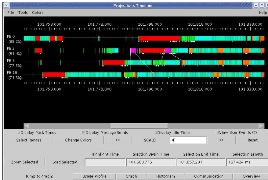
Figure 7.5: NAMD sub-step load balancing with ApoA1 benchmark on Turing
