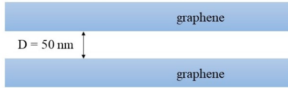
Figure 3.9. Schematic of the problem under study. Two graphene sheets at T = 300 K are separated by a 50 nm vacuum gap.
