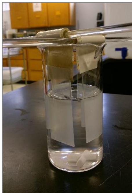
Figure 2.1. Photocatalytic degradation experiment setup; Catalyst coated glass slides immersed in quartz beaker
