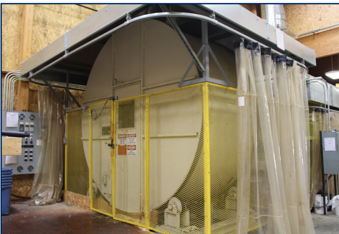
Top: Carmanah Lab Strander, Acrowood and Diamond Roll combination screens; Bottom: One of two Coil spinning disk atomizing resin blenders.
