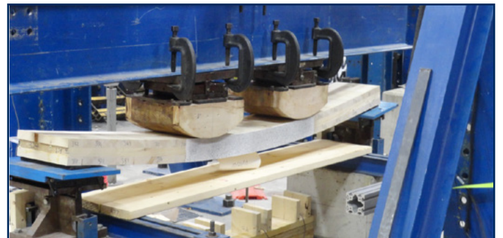
4-point Hybrid CLT Bending Test at UMaine
