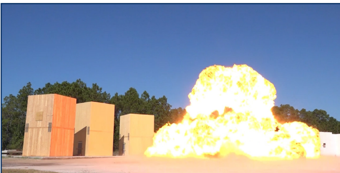
CLT Blast Testing at Tyndall Air Force Base
