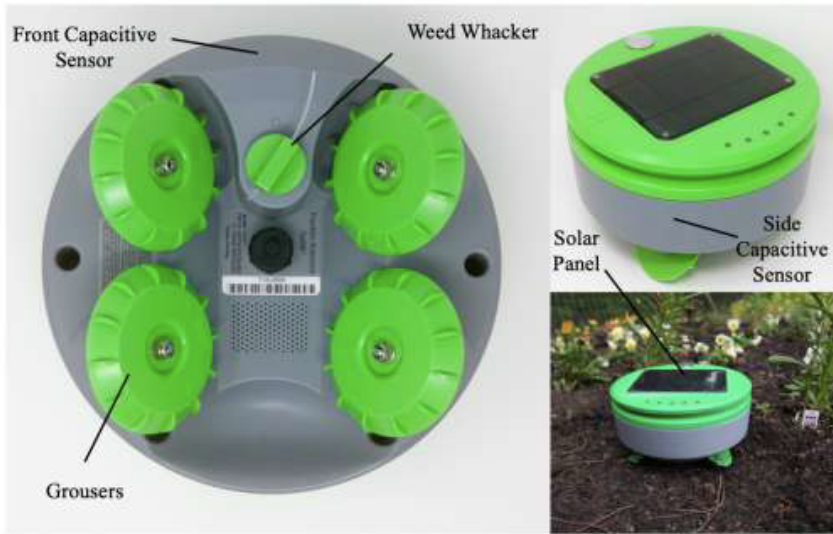
Figure 1.1 Underside of the Tertill™, showing four grousers, weed whacking mechanism, capacitive sensors, and solar panel. Source: Franklin Robotics.
