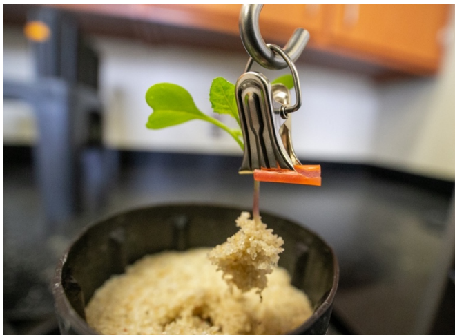
Figure 2.1. A Guillenia flavescens seedling, at one true leaf after being uprooted with an Alluris force gauge.
