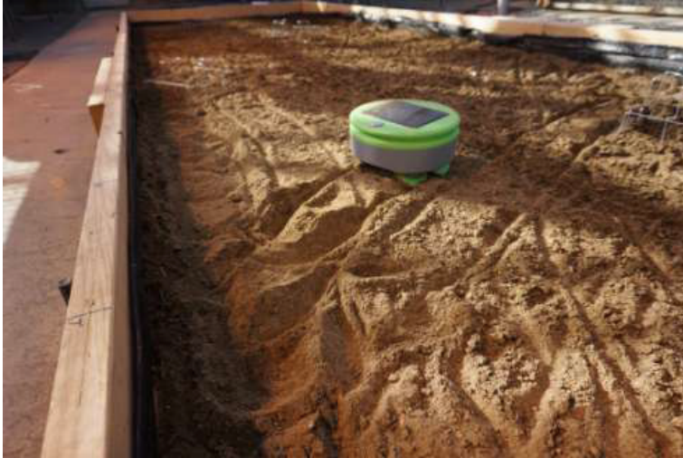
Figure 1.2 Soil disturbance caused by grousers.
