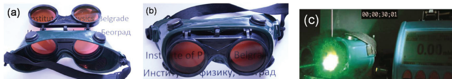
Figure 5. Photograph of TESG eye-protection goggle: (a) for laser adjustment; (b) for laser protection; (c) irradiated with 10W 532nm Nd:YAG laser for 30 s.
