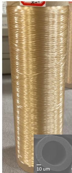
Figure 4.16. A spool of 25 filament HF precursor tow, with inset scanning electron micrograph of a representative HF precursor cross section.
