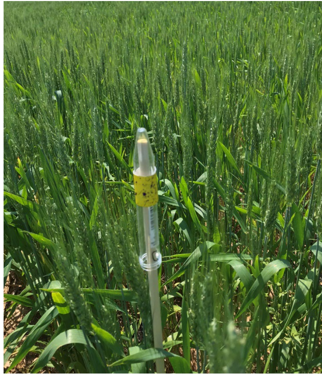
Figure 4.2 Water sensitive paper was wrapped around plastic tubes that were of similar diameter as wheat heads and were placed at the approximate height as surrounding wheat heads. These served as a simulated wheat heads used to measure coverage from different spray nozzle configurations and sprayer speeds in field trials conducted at Princeton, KY in 2017-2019.
