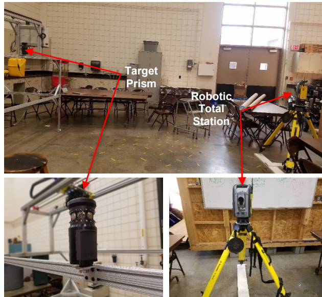
Figure 7: Validation of the linear motion system performance using a robotic total station and target prism. The robotic total station automatically tracked and reported the position of the target prism on a 0.4 s interval.
