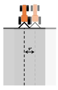
Figure 2. An example of repeatability for two passes over the same swath for two different field operations. The static error is 9 inches.
