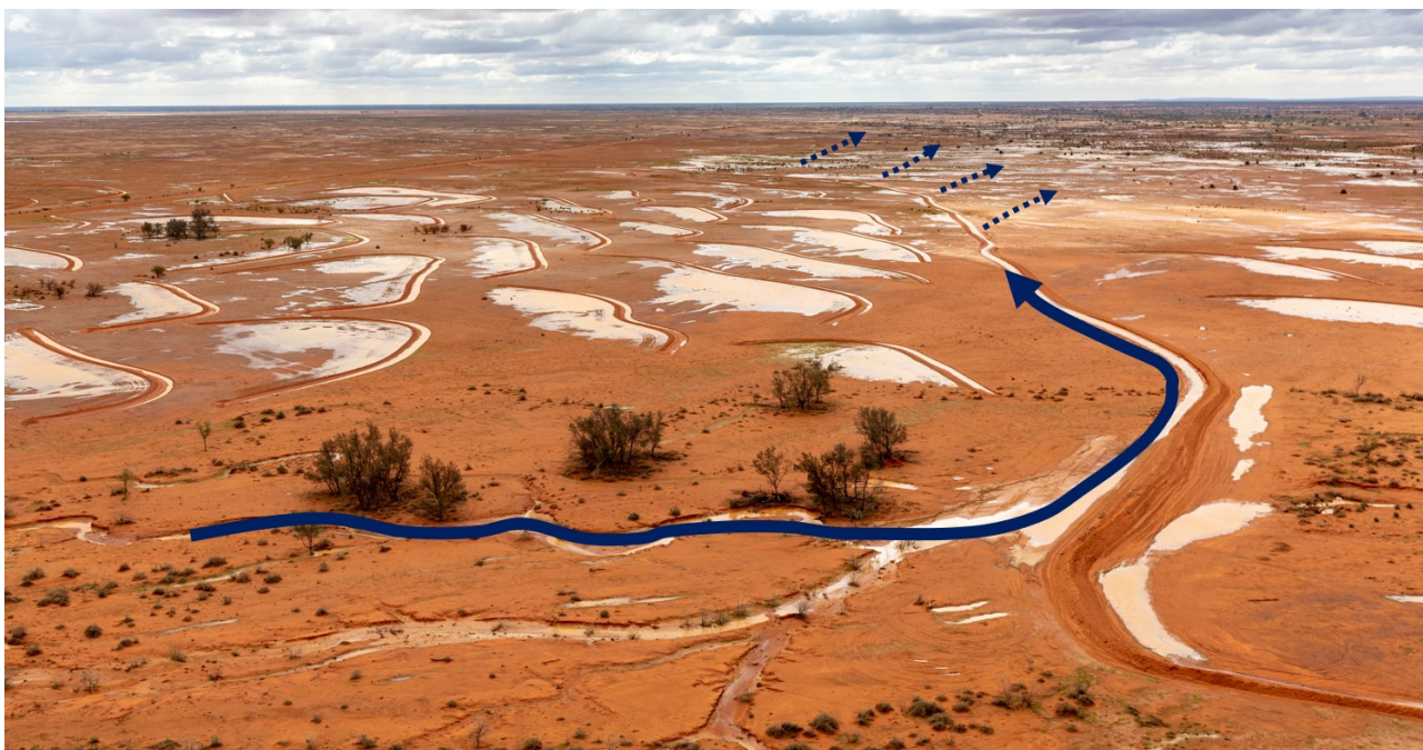
Photo 1: This area shows the critical intervention point of the floodplain rehydration project on Katalpa. Water is diverted out of an erosion gully onto the adjacent floodplain using a diversion bank and deposited via a waterspreading bank. The waterponds (U-shaped banks) rehydrate scalds. This project was identified via the EMU process, with the land manager identifying the critical location and constructing the earthworks. Solid blue arrow indicates concentrated flow; dotted blue arrows indicate low energy flow.
