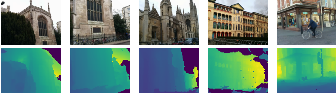
Figure 3.6: Examples of errors in depth labels for Cambridge Landmarks images. Many areas that should have invalid depth are assigned depth values. There are many incorrect depth assignments in general. Dark areas are regions with no depth label (depth=0).
