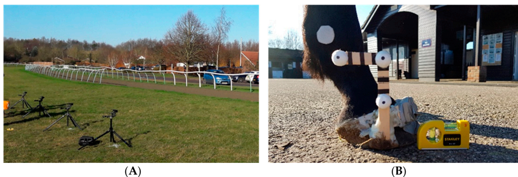
Figure 1. Filming set-up. (A) Four Sony DSC-RX100M5 cameras positioned 8.5 m from the centre of the track and spaced 3.5 m apart. (B) Hoof marker wand used as an aid for tracking hoof orientation through time in video footage.
