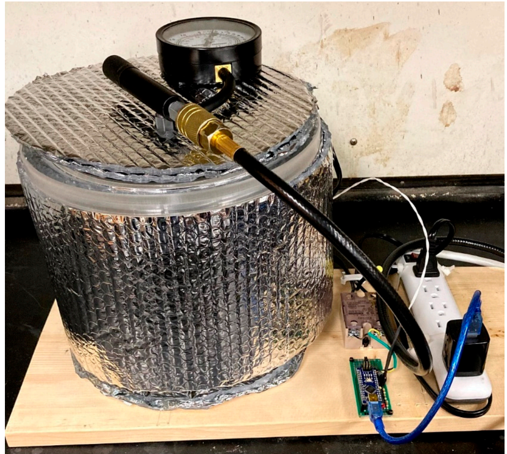
Figure 14. The fully assembled vacuum oven.
