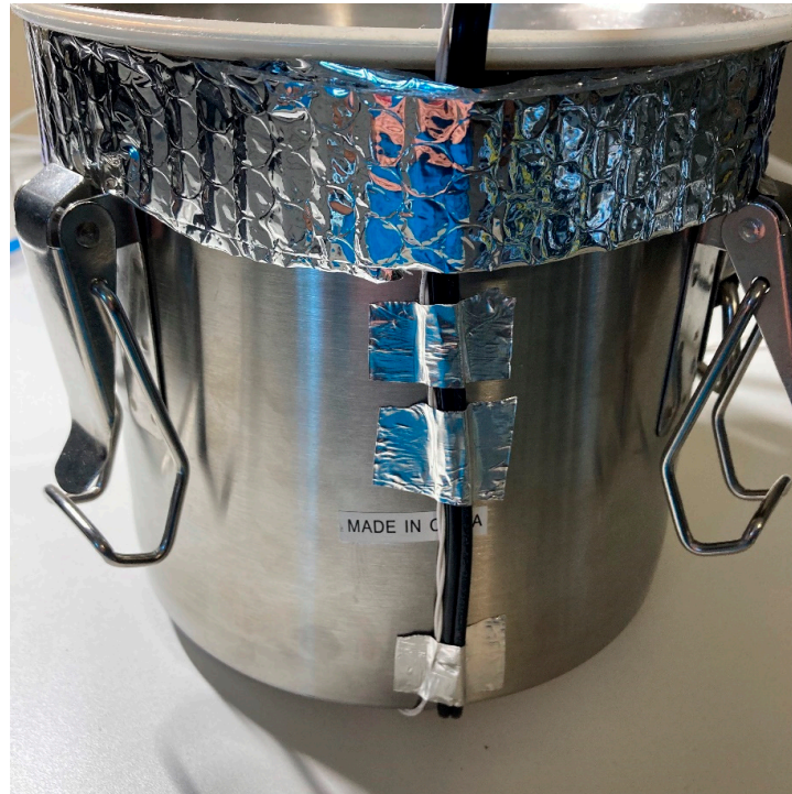
Figure 6. If installed, the heater power cable and sensor wires may be fed up the wall of the chamber for strain relief, but this is not required.
