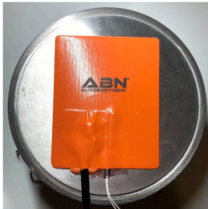
Figure 11. The heating element was adhered to the base of the chamber, with the thermistor secured on the interface.
