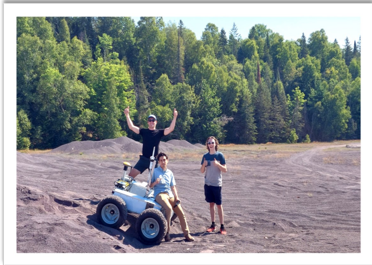
Students in the PSTD test a ground penetrating radar mounted to a robotic mobility platform at the stamp sands. This testing is a part of NASA's LuSTR program where MTU will develop rover-mounted geotechnical and volatile surveying tools to support exploration of the Moon. Photo: Hunter McGillivray
