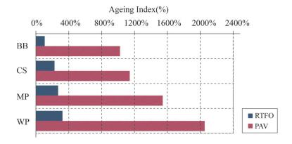
**Figure 5.** Ageing index for complex modulus of RTFO-aged and PAV-aged bio-oil modified asphalts at 64 °C and 10 rad/s [8]. Note: BB refers to swine manure-based bio-asphalt; CS refers to corn stover-based bio-asphalt; MP refers to miscanthus pellets-based bio-asphalt; WP refers to wood pellets-based bio-asphalt.
