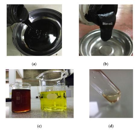
**Figure 3.** Bio-oils derived from various sources: (a) Waste wood [15]; (b) Corn stover [41]; (c) Waste cooking oil [42]; (d) Date seed oil [43].
