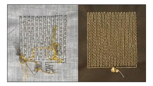
**Figure 4.7:** A comparison between a faulty Resistor with a short circuit (left) and a resistor with proper spaces (right).
