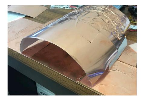
Figure 6.5: Copper tent to provide shielding for the prototype device. Leads to a data acquisition system (DAQ) were attached to the circuit. With the DAQ
