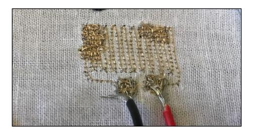
Figure 4.10: Resistor with 4 short circuit pads added to achieve target resistance.
