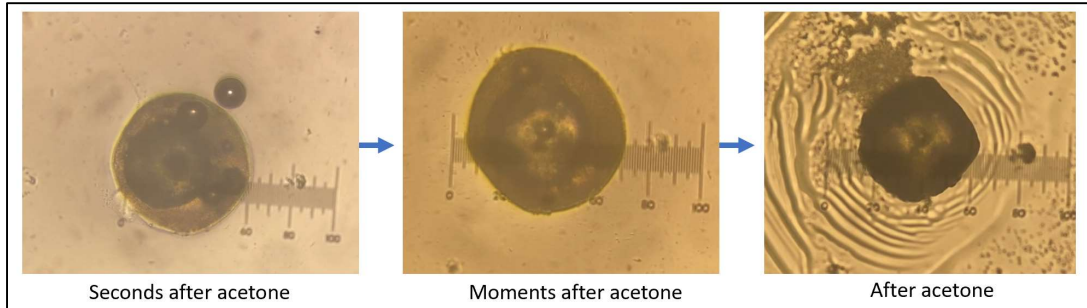
Figure 9. Example images of a double-walled microsphere, fabricated using the double emulsion technique, undergoing dissolution with acetone. The left and center images capture initial and moments after acetone application and the right image captures the final structure of the microsphere after dissolution.
