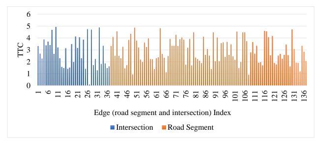
Figure 12 Safety Index (TTC) of different segment of the roads and intersections.
