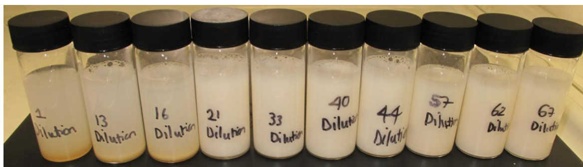
Figure 14. Metolachlor formulations were made based on the triangle points previously demonstrated. The formulations were diluted 1 in 10 in water and left for 30 minutes to check for instability through sedimentation formation.
