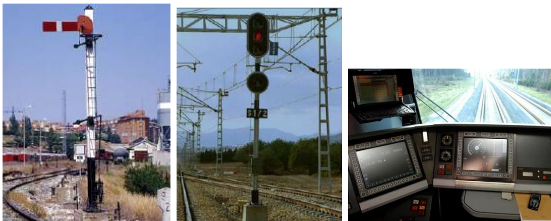
Figure 22: Signalling system examples such as semaphore (shape and colour) and ERTMS (ADIF2008)
