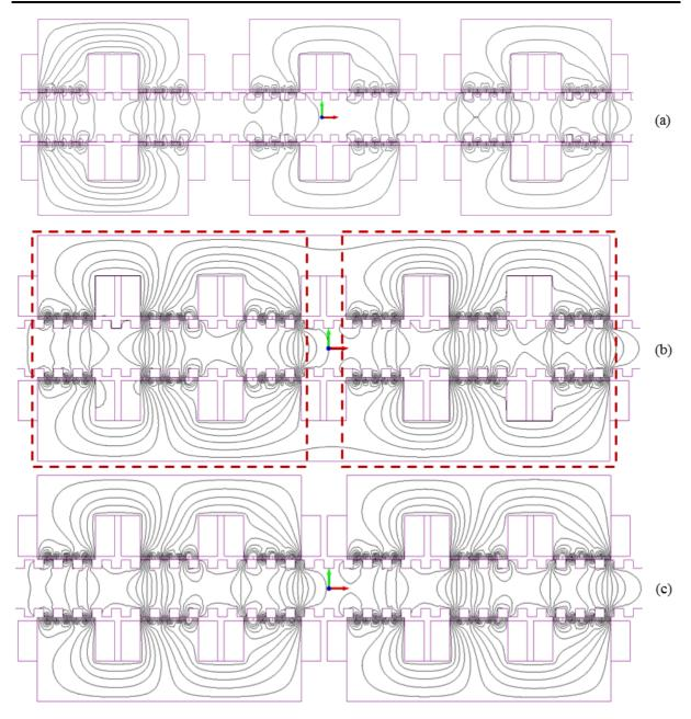
Figure 3. 4: Flux contour plot (a) baseline C-core model (b) integrated core model (c) isolated E-core model
