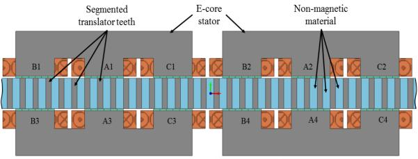
*Figure 3. 13: E-core VHM model with a segmented translator.*
