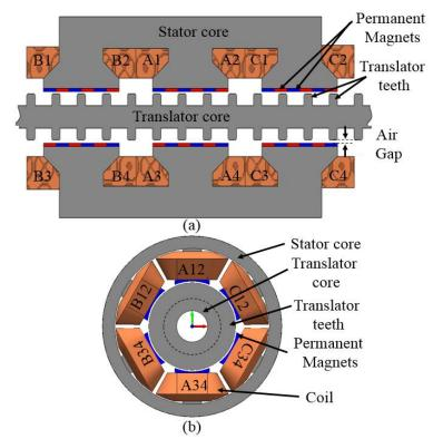
Figure 6. 1: (a) Flat double sided E-core VHM-II (b) cylindrical VHM-II
