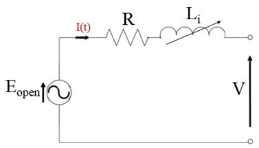
Figure 4. 29: Equivalent circuit model for step variable inductance
