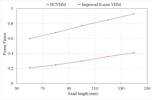
Figure 4. 33: Variation of the power factor with respect to the machine axial length
