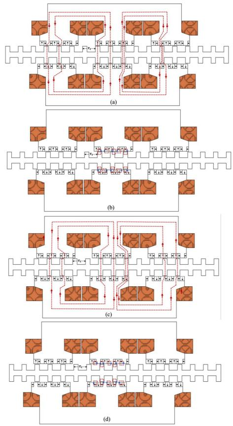
Figure 4. 5: Operation principle at different translator positions (a) Position '0'or '1' (b) Position '1/4' (c) Position '1/2' (d) Position '3/4'.
