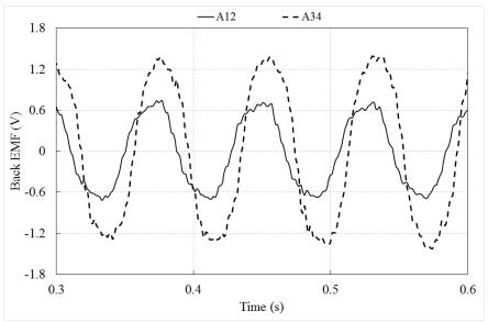
Figure 6. 20: No-load EMF for coil A12 and A34 under phase-A
