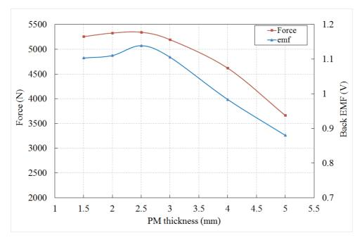
Figure 3. 6: Effect of magnet thickness on back-EMF and average force in the E-core VHM model
