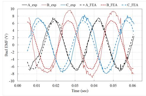
Figure 5. 26: Back EMF comparison between experimental and simulation results over two electrical cycles
