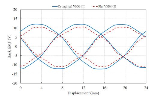
Figure 7. 4: No load three phase back EMF comparison between flat and cylindrical model
