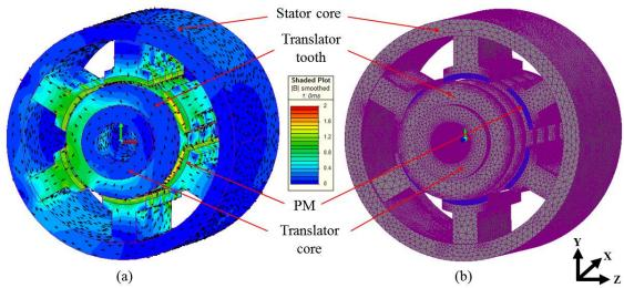
Figure 6. 4: 3D model of cylindrical VHM-II, a) Magnetic flux density distribution b) 3D mesh
