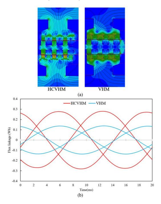
*Figure 4. 4: a) flux contour of the HCVHM and VHM machine b) flux linkage variation between HCVHM and VHM.*
