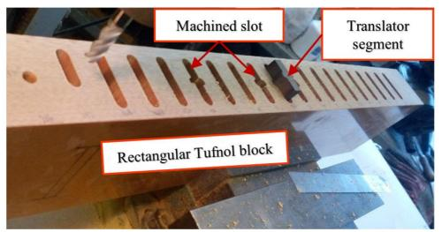
Figure 4. 42: Machining of TUFNOL I-beam structure.
