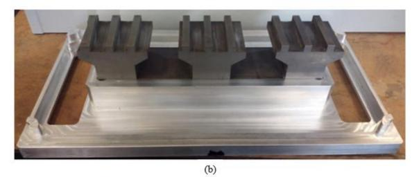
Figure 4. 36: (a) Machining of the aluminium support plate for the stator (b) Stator with aluminium cap support.
