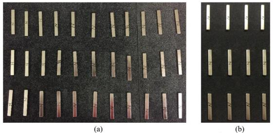
Figure 4. 39: Rectangular Neodymium Iron Boron (N42H) magnets (a) transition magnets (b) Pole magnets
