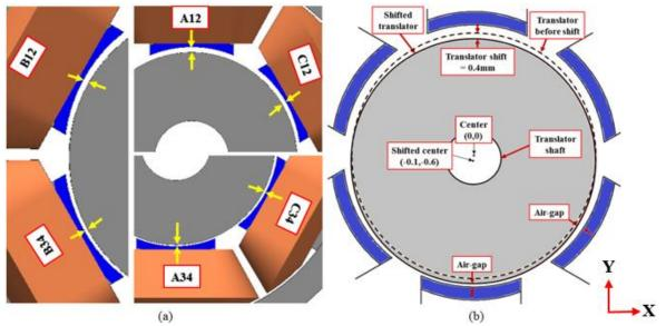
Figure 6. 25: Uneven mechanical air-gap regions (a) simulation (b) geometry.
