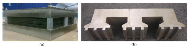
*Figure 4. 34: (a) Lamination stack and bonding structure (b) wire eroded laminated stator*
