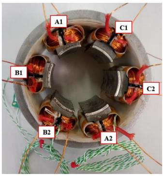
Figure 6. 16: coils assembled stator
