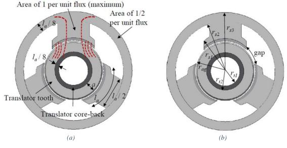
Figure 5. 6: Simple geometry of cylindrical VHM used to build a simple mass model
