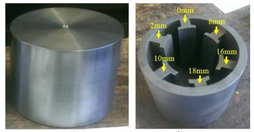
(a) (b) Figure 6. 14: (a) Cylindrical SMC block (b) single piece stator structure
