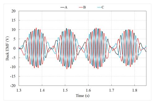
*Figure 6. 26: Measured three phase no load back EMF for three mechanical strokes for linear reciprocating motion, peak linear speed of 1.4m/s.*
