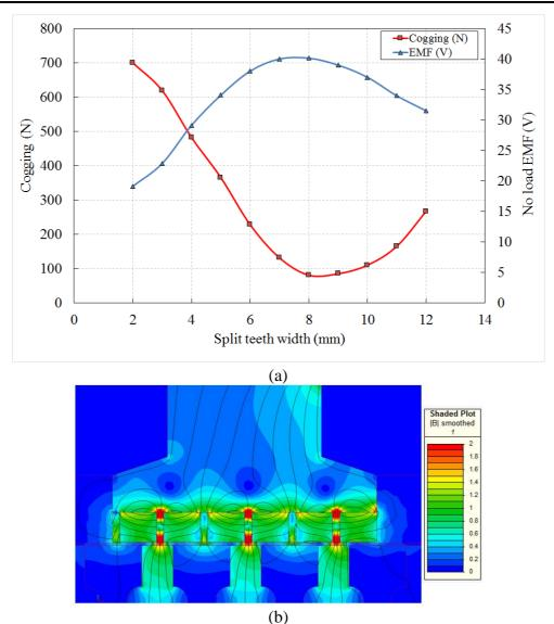
Figure 4.14: a) Cogging and back EMF variation by varying split teeth width b) Flux contour plot at split tooth width of 2mm.
