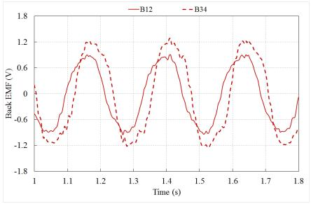
Figure 6. 21: No-load EMF for coil B12 and B34 under phase-B
