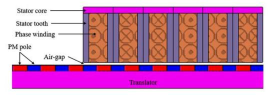
Figure 7. 6: Cross-section of a conventional linear tubular PM machine
