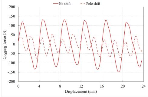
Figure 3. 17: Cogging reduction by implementing lower stator pole shifting
