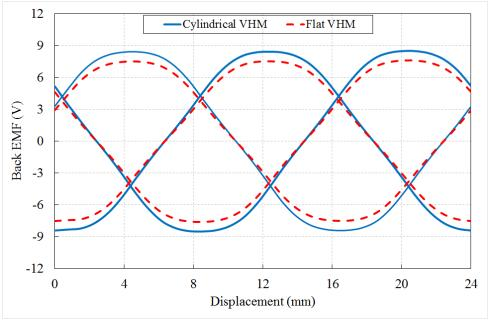
Figure 5. 12: Three back EMF comparison between flat and cylindrical VHM-I
