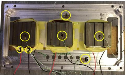
Figure 4. 54: Position of thermocouples on the stator assembly.
