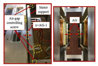
Figure 4. 52: Air-gap controlling by adjustment screws.
