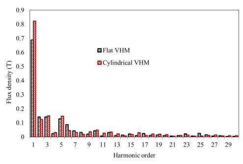
Figure 5. 10: Flux density harmonics comparison for one translator pitch.
