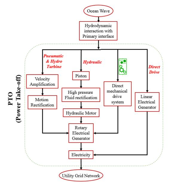
Figure 2. 8: Block diagram of different Power take-off methods
