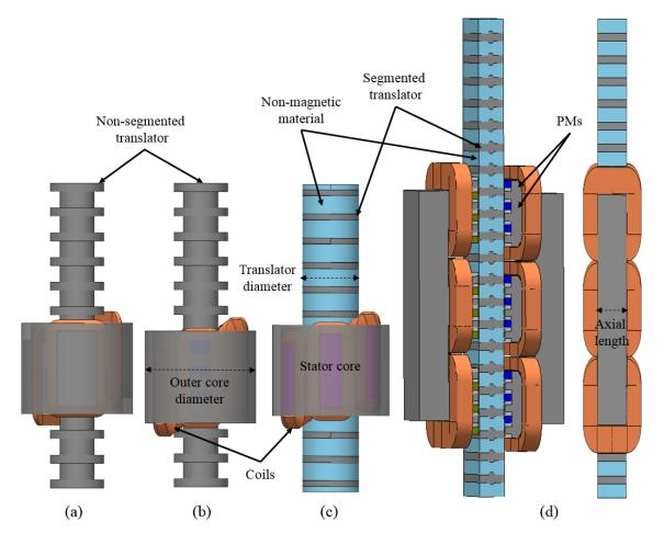
Figure 7. 7: 3D view (a) cylindrical VHM-I with a non-segmented translator (b) Cylindrical VHM-II with a nonsegmented translator (c) Cylindrical HCVHM with a segmented translator (d) flat HCVHM
