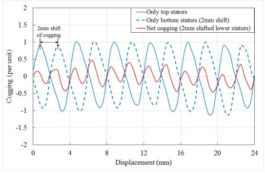
*Figure 3. 18: Cogging reduction technique by shifting lower stators.*
