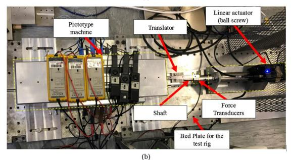
Figure 4. 58: Test rig setup for the prototype machine (a) schematic drawing (b) laboratory assembly
