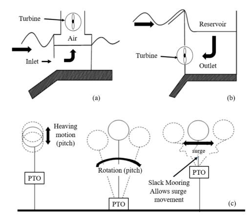
*Figure 2. 5: Classification of Wave Energy Converter (WEC) extraction technologies: (a) oscillating water column, (b) overtopping devices, and (c) oscillating bodies [43, 44]*
