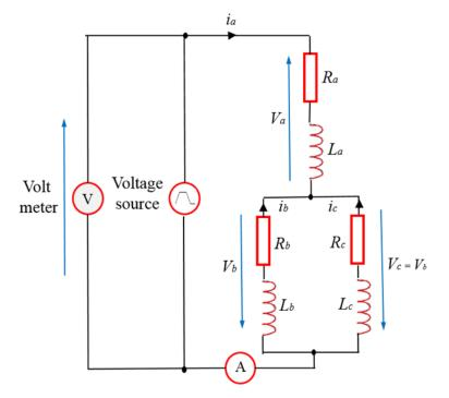
Figure 4. 69: Inductance measurement setup for transient trapezoidal voltage input.
