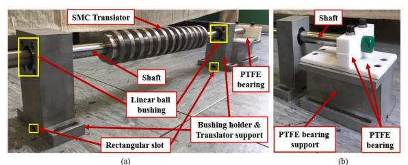
Figure 5. 22: (a) Translator assembly components (b) PTFE bearing support and end cap bearings.
