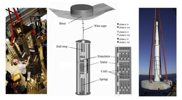
Figure 2. 11: On the left, the inside of the converter of Seabased AB. On the center, floating buoy with the WEC device and a detail of the excitation winding system. On the right, the real prototype of the WEC device[60]
