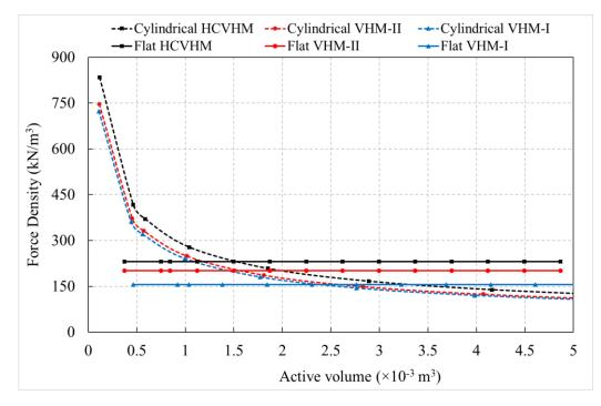
Figure 7. 10: Force density against equivalent axial length plot for all six machine topologies.
