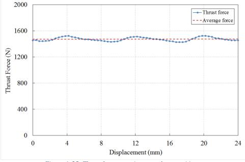
Figure 4. 25: Thrust force at various translator positions.
