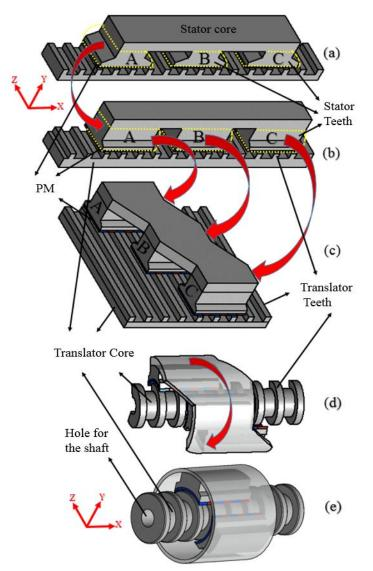
Figure 5. 3: Cylindrical VHM-I model development from flat VHM-I
