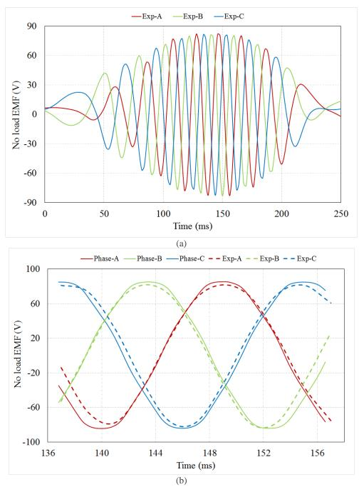
Figure 4. 65: Measured no-load EMF at variable speed (a) for single mechanical stroke (b) compared with simulation over one electrical cycle.
