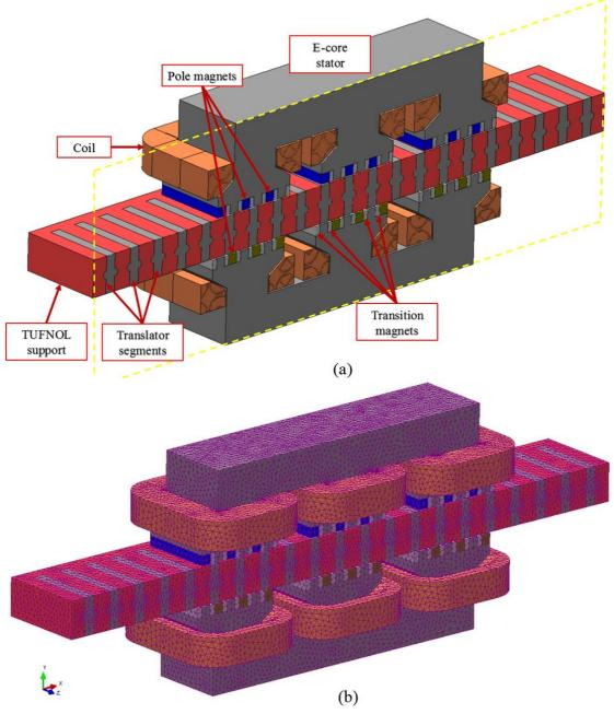
Figure 4. 17: (a) Final 3D model with segmented translator (b) 3D mesh.
