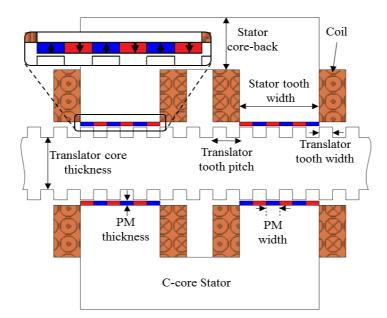
Figure 3. 1: Single phase of the baseline C-core double sided Vernier Hybrid Machine
