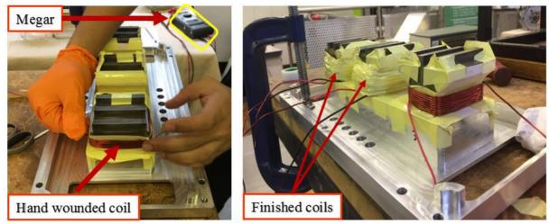
Figure 4. 38: Hand wounding process and finished coils.
