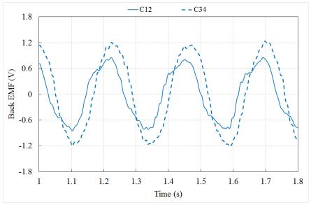
Figure 6. 22: No-load EMF for coil C12 and C34 under phase-C
