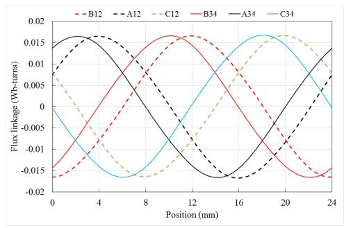
Figure 6. 8: No load armature coil flux linkage
