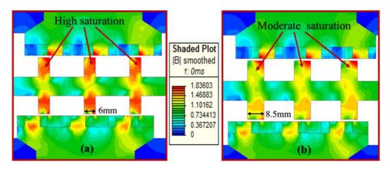
Figure 4. 9: Effect of magnetic flux saturation on translator teeth at rated current (a) 6mm (b) 8.5mm
