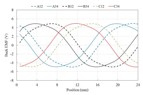
Figure 6. 9: No load armature coil back EMF
