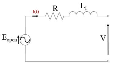
Figure 4. 26: Simple per phase equivalent circuit
