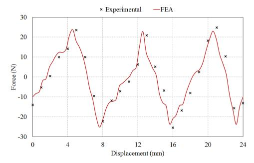
Figure 4. 59: Cogging force variation with the translator displacement after removing offset.
