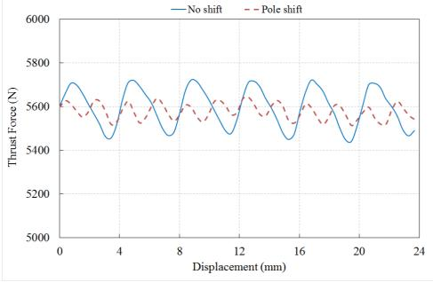
Figure 3. 19: Thrust force comparison between shifted and non-shifted lower stator.
