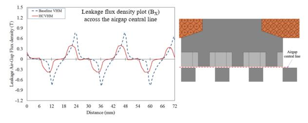
Figure 4. 19: Leakage air gap flux density  $(B_X)$  comparison
