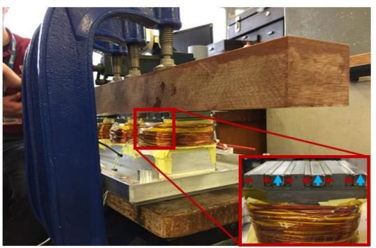
Figure 4. 40: Magnet assembly and curing stage in a stator.
