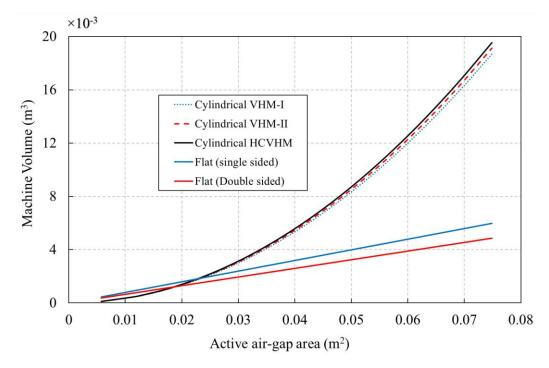
Figure 7. 9: Comparison of active machine volume with different topologies of cylindrical and flat machines for fixed axial length, copper mass, and magnet mass
