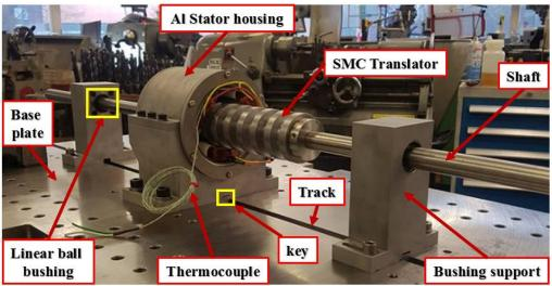
Figure 5. 23: Final Machine assembly on the bed plate.
