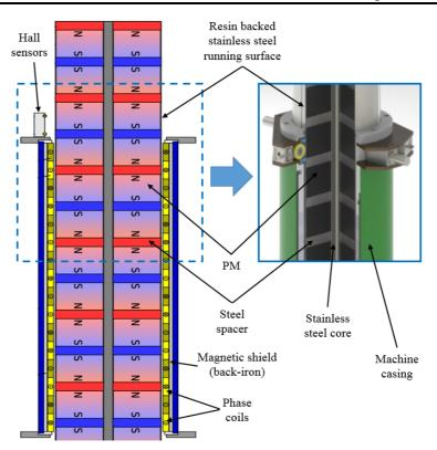
Figure 2. 13: Schematics details of the slot-less linear generator for the converters of Trident Energy being installed for testing at the sea [64-66]
