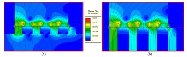
Figure 3. 11: Flux density plot under phase-A a) translator with core back b) segmented translator
