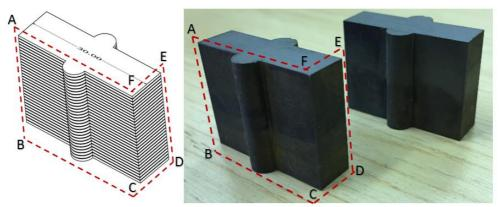
Figure 4. 41: Segmented translator teeth from laminated steel.
