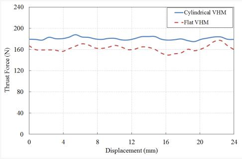
Figure 5. 15: Thrust force comparison between flat and cylindrical VHM-I
