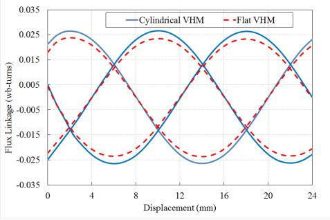
Figure 5. 11: Three flux linkage comparison between flat and cylindrical VHM-I
