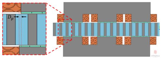
*Figure 3.15: Lower stator shifted model to reduce cogging.*
