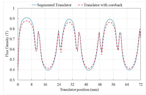
Figure 3. 12: Flux density comparison of the E-core VHM between the cored and coreless translator
