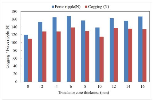
Figure 4. 13: Cogging and force ripple variation by varying translator core thickness.
