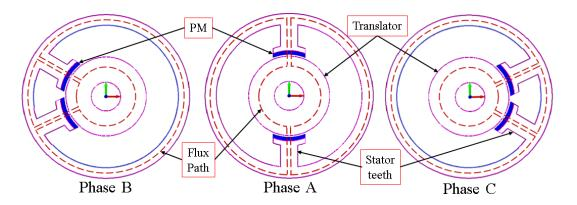
Figure 6. 3: 2D flux path representation of the separated three phases of the cylindrical machine
