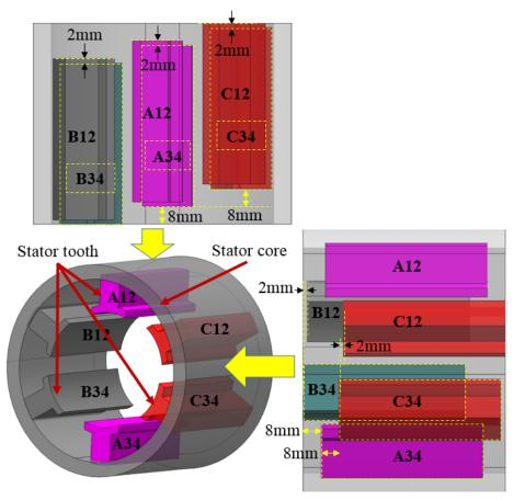
Figure 6. 5: Stator teeth geometry of the cylindrical topology for cogging reduction
