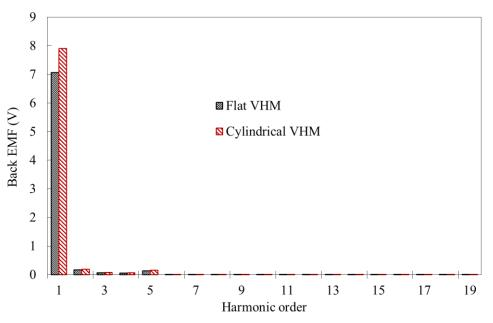
Figure 5. 13: Back EMF harmonics of flat and cylindrical VHM-I
