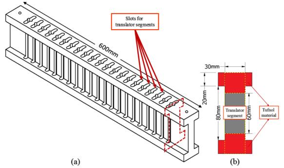
*Figure 4. 43: (a) Machined TUFNOL I-beam structure with slots for translator segments (b) cross-section of the slot.*
