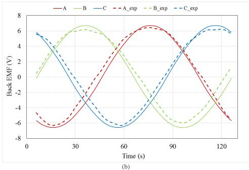
Figure 4. 64: Measured no-load EMF results (a) AG=1mm (b) AG=2mm.
