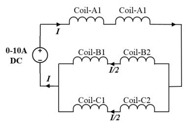
Figure 4. 60: Electrical circuit connection for the static force measurement.
