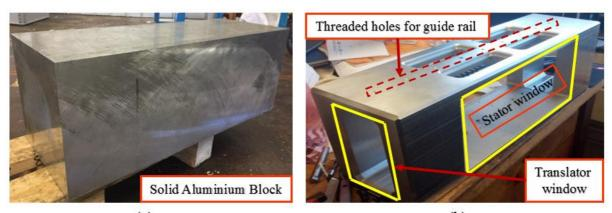
(a) (b) Figure 4. 50: Aluminium housing (a) solid Aluminium block (b) machined structure.
