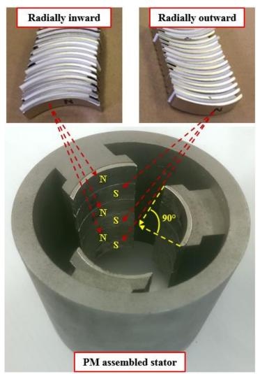
Figure 5. 18: Arc-shaped PMs and magnet assembled stator
