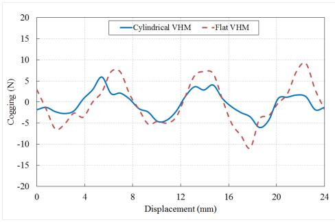
Figure 5. 14: Cogging force comparison between flat and cylindrical VHM-I
