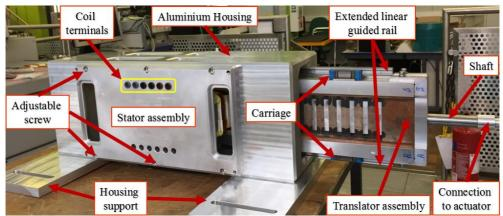
Figure 4. 53: Fully assembled linear HCVHM with segmented translator
