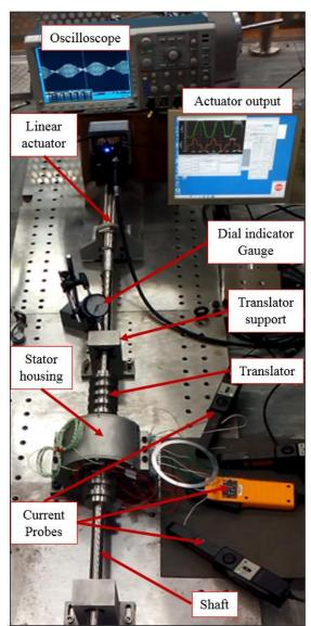
Figure 6. 19: Prototype cylindrical VHM-II is driven by a ball screw actuator and being tested.
