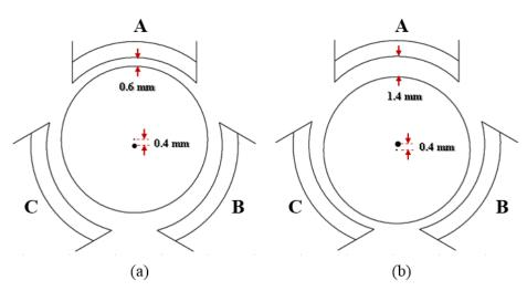
Figure 5. 28: Air-gap imbalance (a) translator shifted up by 0.4mm (b) translator shifted down by 0.4mm
