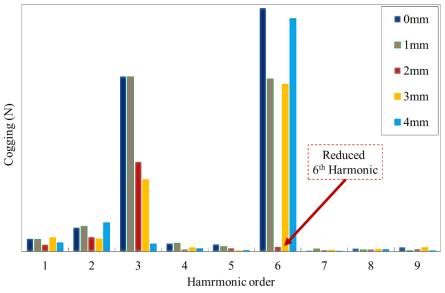
Figure 6. 6: Harmonic distribution for different pole shifted models.
