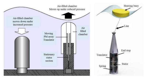
Figure 2. 7: On the left: Schematic of a converter AWS. On the right: converter with concept Seabased AB. Both use a linear generator as a way of taking power.
