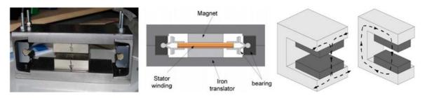
*Figure 2. 14: On the left, a module of translator C-Gen. In the centre, characterisation of the module. On the right, the distribution of the magnetic flow lines in a module [67].*
