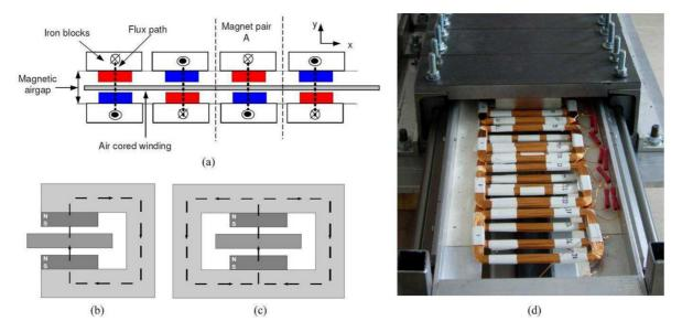
Figure 2. 15: 2D Schematic diagram between modules of the linear generator, C-Gen a) Double-sided generator with magnet pairs separated into modules (b)&(c) magnetic flux distribution in a module (d) coil mounted on the c-core module [67]
