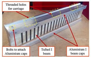
Figure 4. 46: Attaching the aluminium I-beam caps on the TUFNOL Structure.
