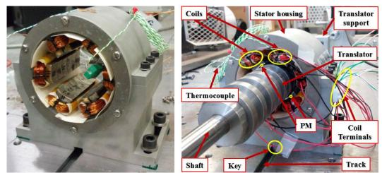
Figure 6. 18: Assembled stator on the bed plate and the full machine assembly.
