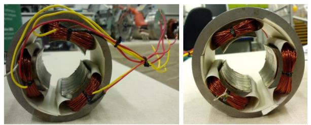
Figure 5. 19: Completed three phase windings in the stator
