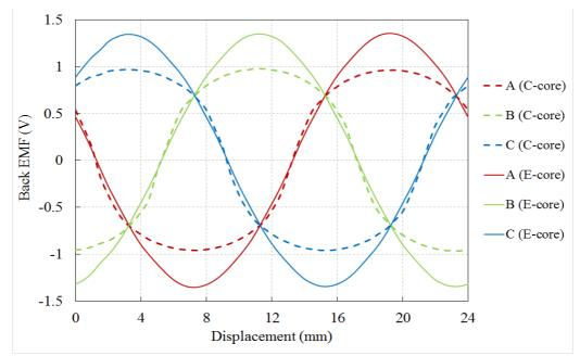
Figure 3. 21: Back-EMF comparison between C-core baseline model and the optimised E-core model over an electrical cycle.
