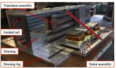
Figure 4. 51: Assembling the translator and the stators in the aluminium housing
