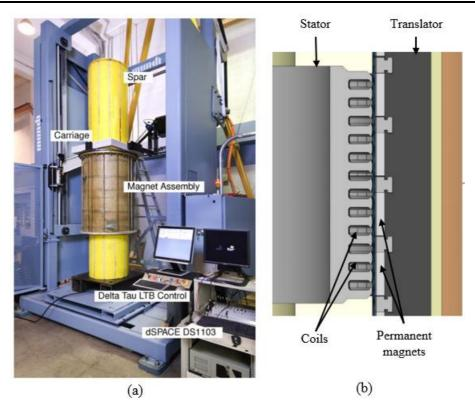
*Figure 2. 12: (a) SeaBeav-I with integrated permanent magnet linear generator on the linear test bed [63] (b)* 2D crossectional view of the generator component [61]
