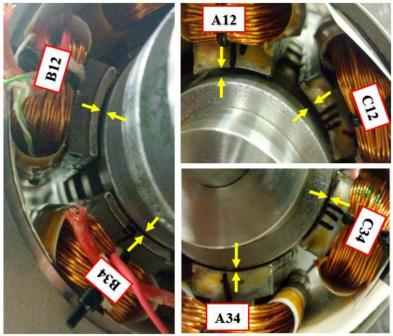
Figure 6. 24: Uneven mechanical air-gap regions of the prototype.
