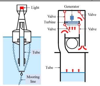
Figure 2. 1: Outline of Japanese navigation buoy equipped with air turbine [15]
