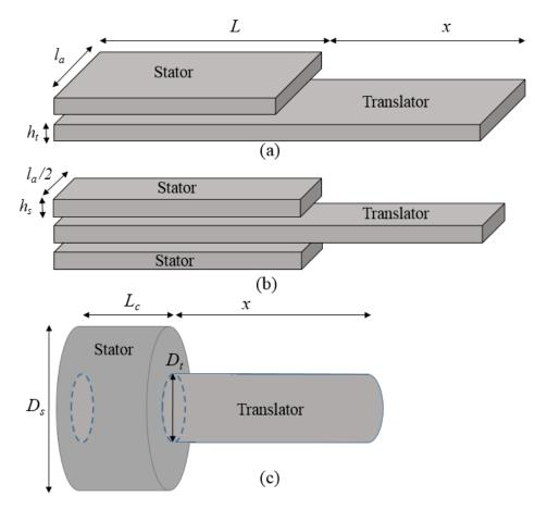
*Figure 7. 8: General linear machine dimensions, including stroke length, x (a) Single sided flat topology (b) double-sided flat topology with a shorter axial length (c) Cylindrical topology.*
