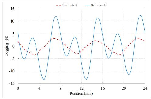
Figure 6. 7: Cogging force variation by pole shifting.
