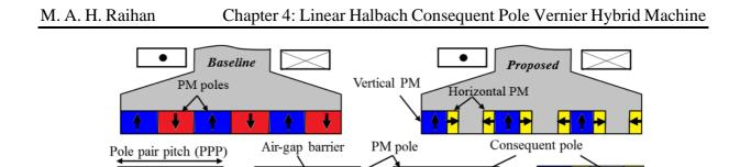
PM array development Figure 4. 2: Schematics of PM array development of proposed HCVHM machine from baseline VHM.
