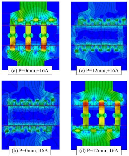
Figure 4. 22: Flux contour plot at different translator position at different DC excitation current.
