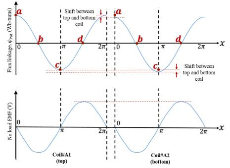
*Figure 4. 6: Single phase no-load flux linkage and back EMF of the top and bottom stator coils under the same phase.*
