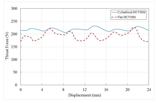
Figure 7. 5: Electromagnetic thrust force comparison between flat and cylindrical model
