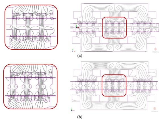
Figure 4. 11: No load flux contour path of HCVHM (a) solid translator (b) segmented Translator
