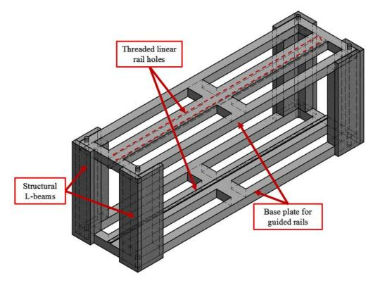
Figure 4. 48: Initial design for the steel housing structure
