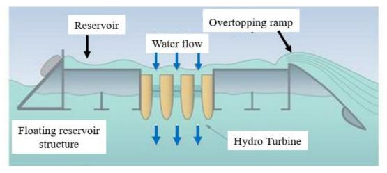
Figure 2. 6: Principle of operation of an Overtopping system (Wave Dragon).
