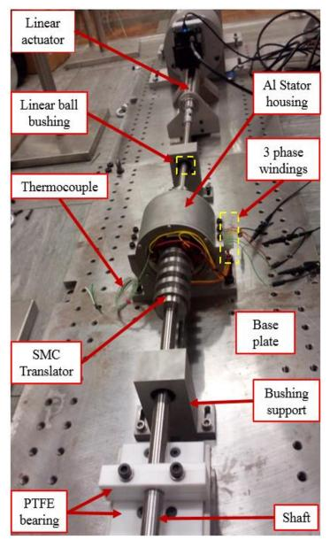
Figure 5. 24: Fully assembled cylindrical VHM-I mounted on the test rig.
