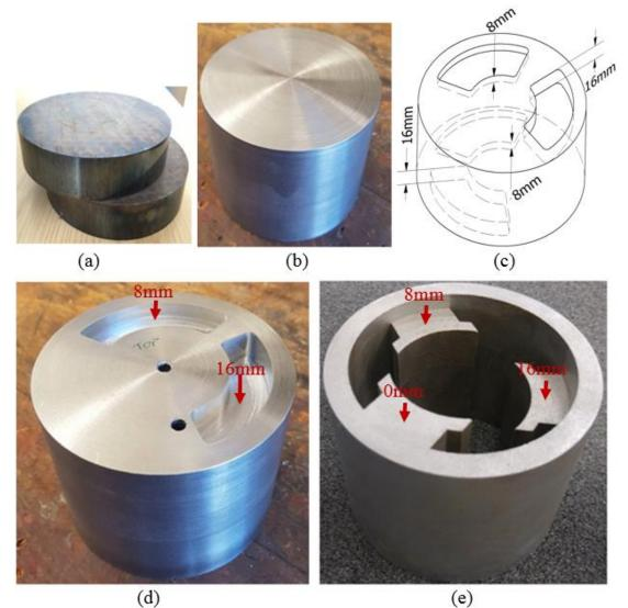
Figure 5. 17: Cylindrical SMC stator construction processes
