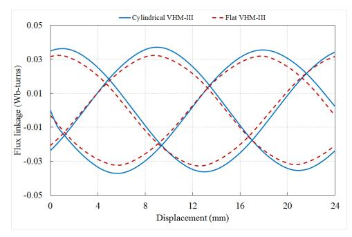
Figure 7. 3: No load magnetic flux linkage comparison between flat and cylindrical model
