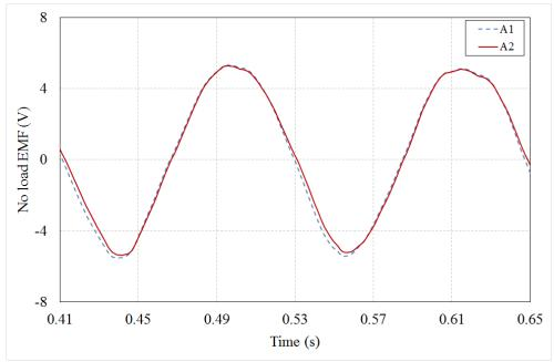
Figure 4. 63: Measured no-load EMF for two coils under the same phase at 0.2m/s
