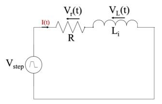
*Figure 4. 30: Simple per phase equivalent circuit model with a trapezoidal DC voltage source*
