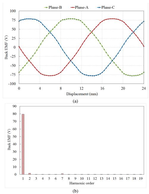
Figure 4. 20: a) Three phase back EMF for the proposed HCVHM. b) Harmonic analysis of phase back EMF.
