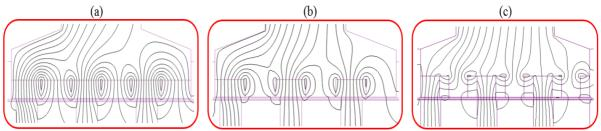
Figure 4. 3: Magnetic flux contour under stator pole a) VHM b) Consequent Pole VHM c) HCVHM topology
