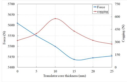
Figure 3. 10: Translator core thickness optimisation in terms of average force and cogging
