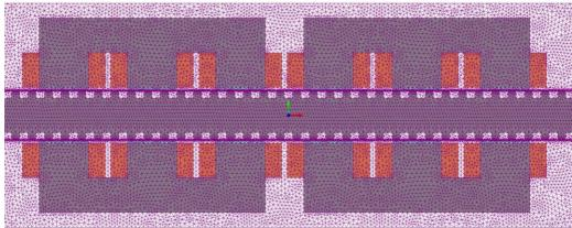
Figure 3. 5: Refined 2D mesh for the E-core model.
