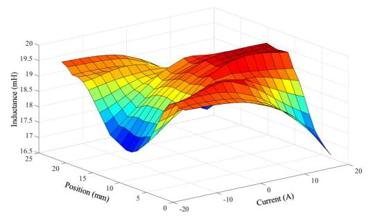
Figure 4. 28: Self-inductance at a different position for different current levels.
