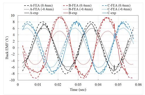
Figure 5. 29: Measured (exp) and simulated (FEA) results for two values of offset translator.
