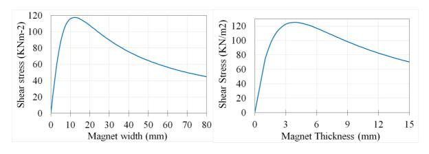
Figure 3. 2: Analytical analysis of Magnet Thickness and width for maximum shear stress on the baseline VHPM machine.
