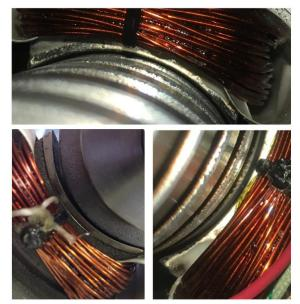
Figure 5. 27: The three air-gap regions of the prototype under three stator teeth.
