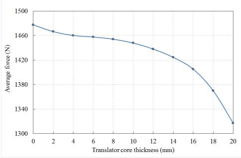
Figure 4. 12: Average force and back EMF variation by varying translator core thickness.
