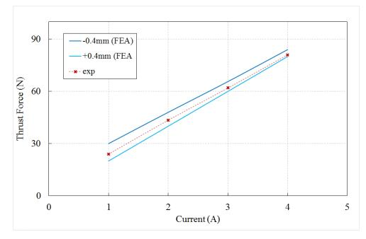
Figure 5. 32: Peak force comparison between simulation and experimental results for varying current.
