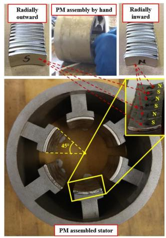
Figure 6. 15: PM assembly and the stator.
