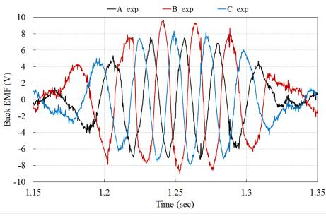
Figure 5. 25: Measured EMF for single mechanical stroke.
