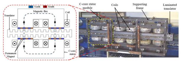
Figure 2. 17: The 3kW prototype VHM generator and the 2D cross-section of a C-core unit [7]
