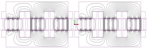
Figure 3. 14: No load flux contour plot for the E-core VHM model with the segmented translator
