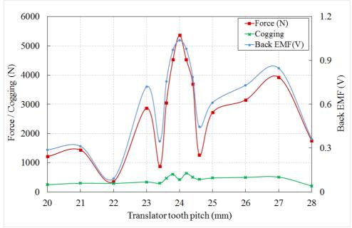
Figure 3. 8: Translator tooth pitch analysis with equal tooth and slot
