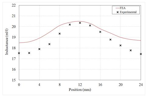
Figure 4. 68: Comparison of experimental and simulation predicted self-inductance of an entire phase.
