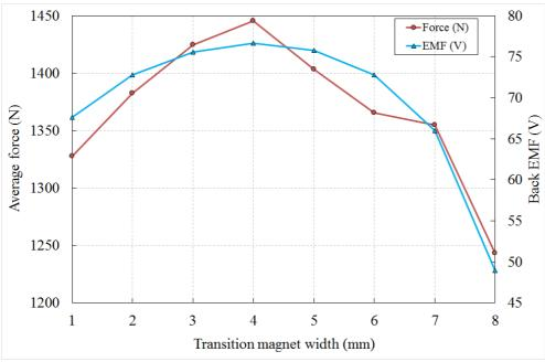
Figure 4. 15: Average force and back EMF variation with the transition PM width.
