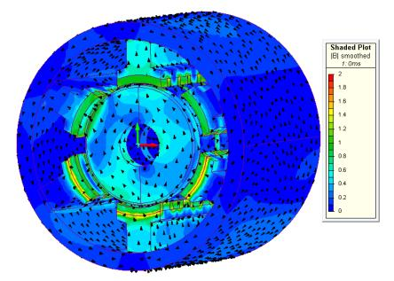
Figure 7. 2: No load magnetic flux distribution plot of the cylindrical HCVHM
