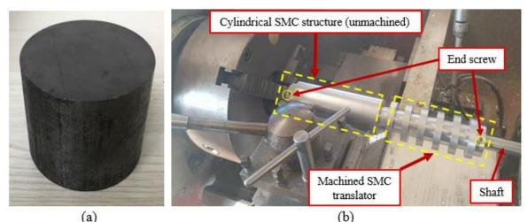
Figure 5. 21: (a) 40mm long SMC block (b) translator construction in the milling machine.
