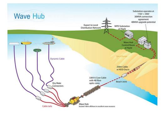
*Figure 2. 3: Wave Hub - Infrastructure for development and testing of wave energy converters in Cornwall – England* [28].
