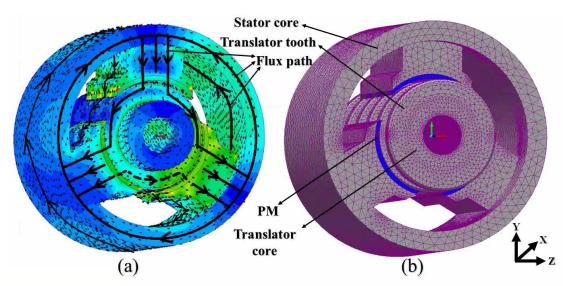
Figure 5. 8: The cylindrical prototype design in 3D FEA, a) magnetic flux distribution and b) 3D mesh
