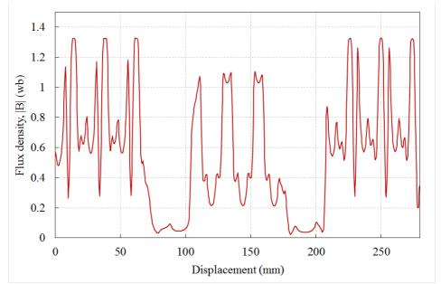
Figure 4. 18: Active air gap flux density of the HCVHM model over the active machine length.
