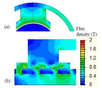
Figure 5. 7: Equivalence of flux density in the stator core back for (a) Cylindrical VHM-I (b) Flat VHM-I
