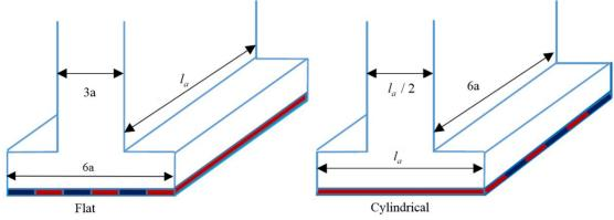
Figure 5. 5: Simple geometry of flat VHM used to build a simple mass model.
