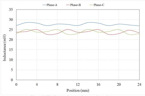
Figure 4. 32: Phase inductance between three phases.
