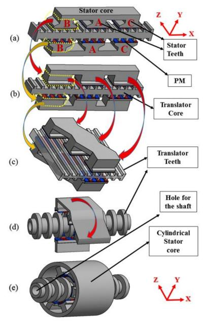
Figure 6. 2: Cylindrical Vernier machine topology development.
