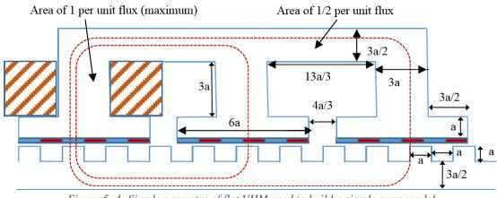
Figure 5. 4: Simple geometry of flat VHM used to build a simple mass model
