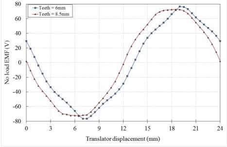
Figure 4. 10: Phase-A back EMF for different translator teeth width
