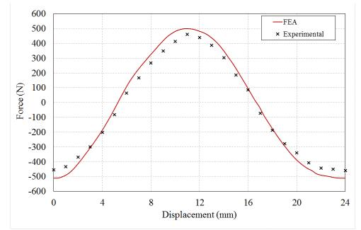
Figure 4. 62: Static force test at different translator position during 8A DC excitation (air-gap=2mm)
