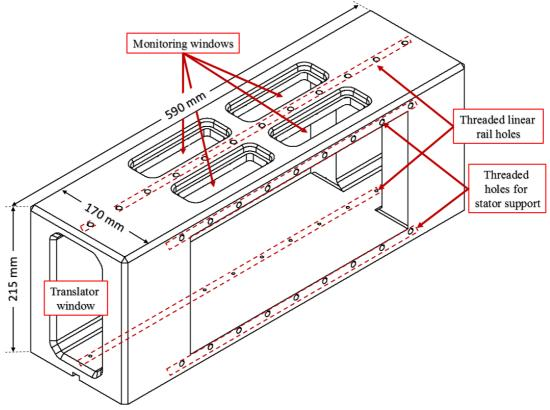
Figure 4. 49: Final design of the aluminium housing.
