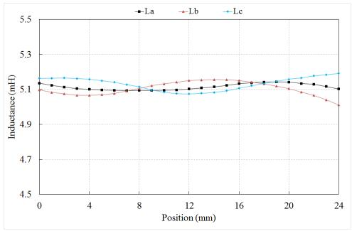
Figure 5. 16: Three phase inductance of the cylindrical machine.
