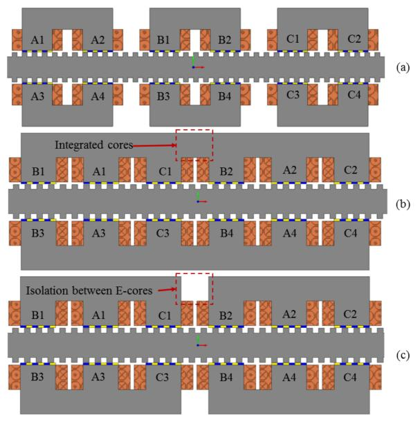
Figure 3. 3: Three phase VHM a) Initial C-core design b) Modified integrated core design c) Isolated E-core design
