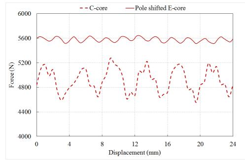
*Figure 3. 22: Average thrust force comparison between C-core baseline and improved the E-core VHM models over an electrical cycle.*
