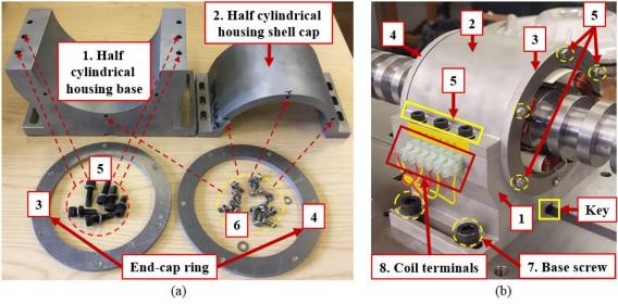
Figure 5. 20: (a) Stator housing components (b) stator assembly.
