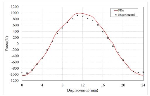
Figure 4. 61: Static force test at different translator position during 8A DC excitation (air-gap=1mm)
