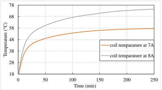
Figure 4. 56: Temperature rise of the coil center at different DC current level.
