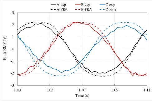
Figure 6. 23: Three-phase EMF comparison between measured and predicted results
