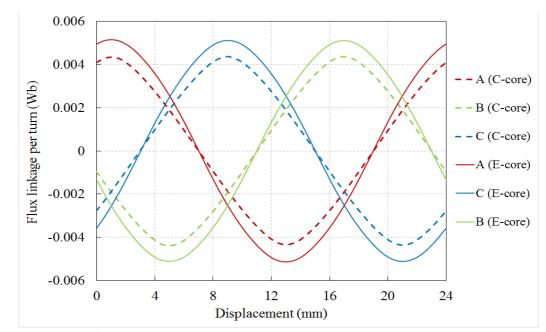
*Figure 3. 20: No load flux linkage comparison between C-core baseline model and the optimised E-core model with the segmented translator over an electrical cycle.*
