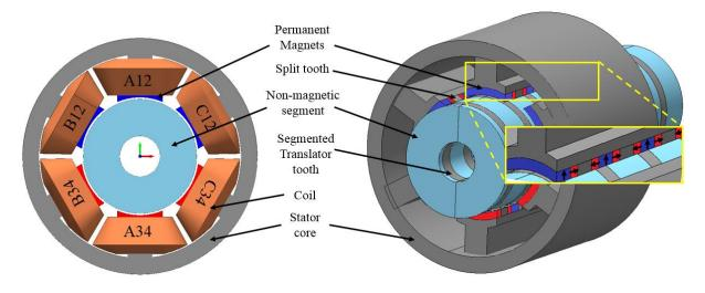
Figure 7. 1: Cylindrical Halbach Consequent Pole VHM
