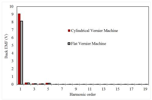
Figure 6. 11: EMF harmonics comparison between flat and cylindrical
