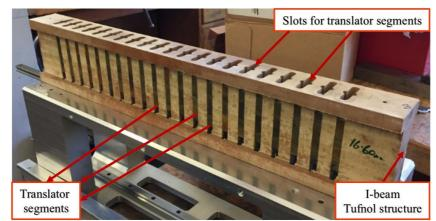
Figure 4. 44: Assembly of translator teeth segments inside the TUFNOL I-beam structure.
