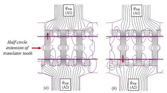
*Figure 4. 7: No load flux contour plot with a segmented translator (a) translator teeth align with pole magnets of the top stator (b) translator teeth align with pole magnets of the bottom stator.*
