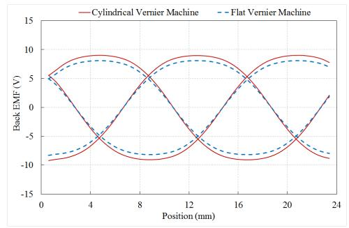
Figure 6. 10: Three-phase back EMF comparison between flat and cylindrical topology
