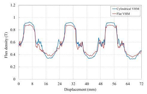
Figure 5. 9: Flux density comparison under full stator tooth length during maximum flux linkage
