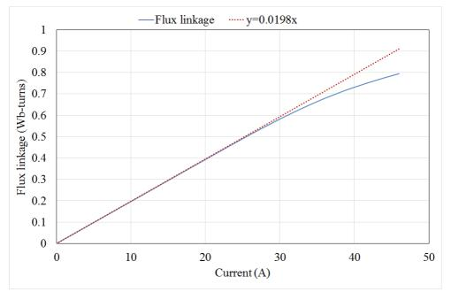
Figure 4. 27: Variation of phase flux linkage with only excitation current, without magnetic excitation.
