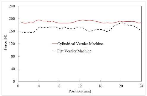
Figure 6. 12: Thrust force comparison between flat and cylindrical VHM-II at rated current
