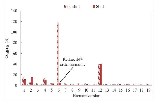
Figure 3. 16: Harmonic analysis of cogging force between shifted and non-shifted lower stator model.
