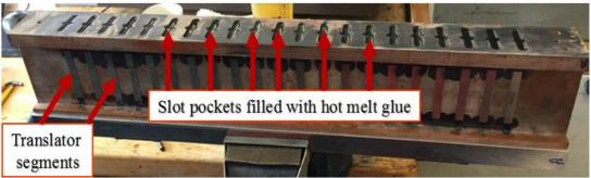
Figure 4. 45: Assembly of the translator teeth segments inside the TUFNOL I-beam structure.
