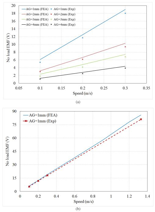
Figure 4. 66: Measured no-load EMF variation with speed (a) different air-gap (b) at 1mm air-gap.
