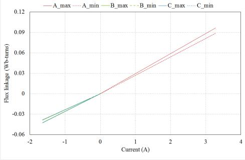
Figure 4. 70: Flux linkage plots against the current for three phases.
