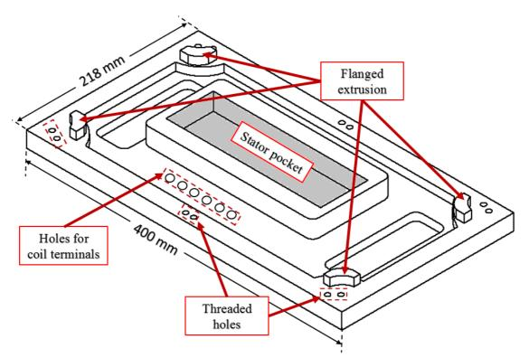
Figure 4. 35: Aluminium support structure for the stator assembly.
