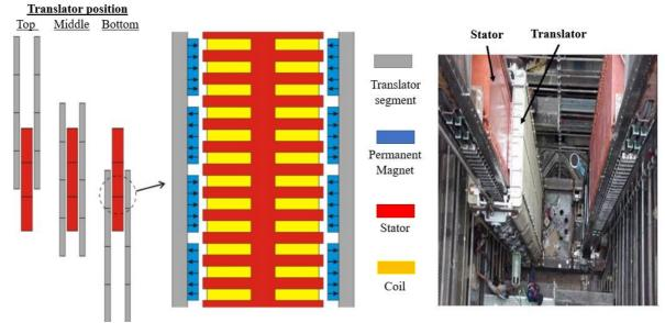
Figure 2. 10: AWS linear generator topology and its translator assembly.[27, 47]
