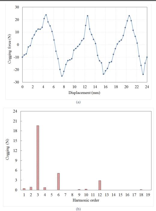
Figure 4. 23: (a) Cogging force for the final design (b) harmonic analysis of the cogging force.
