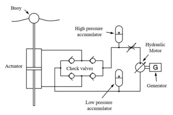
Figure 2. 9: Hydraulic PTO system for wave energy conversion [22]
