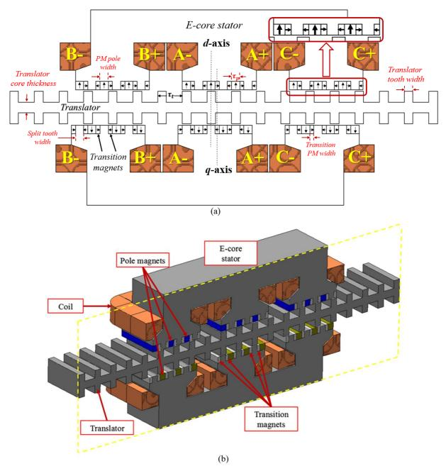
Figure 4. 1: Proposed HCVHM with magnet orientation and three phase windings (a) 2D (b) 3D cross section
