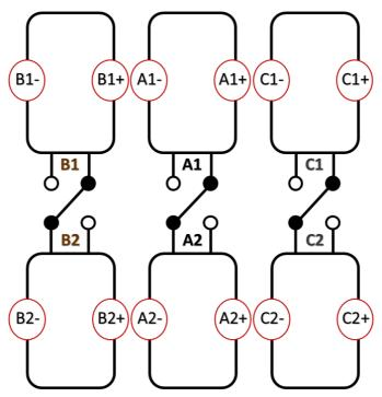
Figure 4. 37: Winding configuration for top and bottom stator
