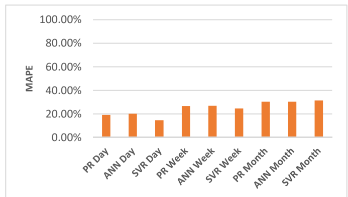
(b) A comparison of the MAPEs of predicting summer building energy usage with PR, ANN and SVR.
