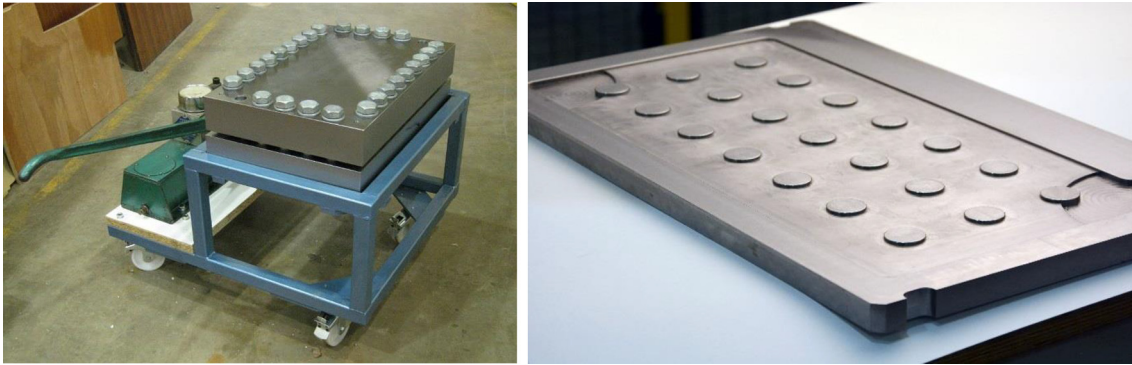
Fig. 8. (a) The hydroforming facility, (b) the mould plate. The surface seen here faces downwards in the facility.
